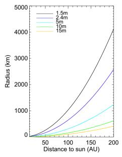
**Fig. 2** Minimal radius of the observable KBOs as a function of the distance to the Sun, to have a count rate of 100 for 10 min of observation, assuming the instrumental efficiency of HST/COS and a Lambertian albedo of 0.5 in the 260–310 nm spectral range, for different telescope aperture diameter
