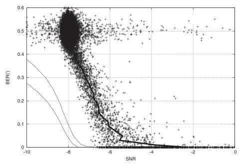
**Fig. 7.** A figure showing the preliminary results of the spread spectrum based data transmission system. A scatter plot of the Signal to Noise Ratio plotted against the Bit Error Rate (BER) measured in 320-bit bursts is depicted. Every cross corresponds to a single experiment.
