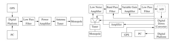
**Fig. 5.** Transmitter (left frame) and receiver (right frame) used for sounding and data transmission on the HF link. We note that the full transceiver is mainly digital, with only some filtering, amplification and antenna tuning performed in the analog domain.
