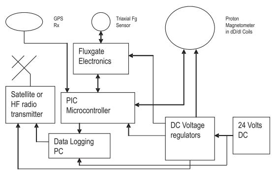
Fig. 2. Block diagram of the new station.
