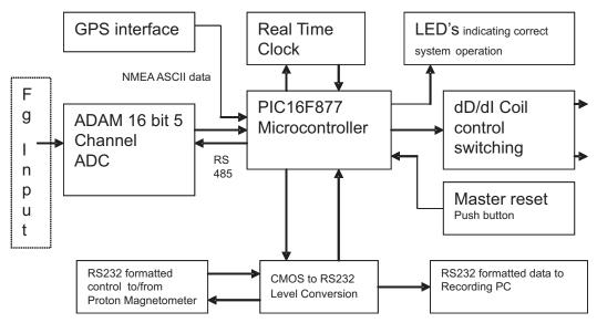
Fig. 3. Controller Block Diagram.
