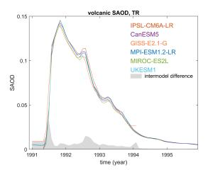
**Figure 1.** Monthly-mean aerosol optical depth at 550 nm due to stratospheric volcanic aerosols (variable aod550volso4) averaged over the tropics  $(30^{\circ} \text{ S}-30^{\circ} \text{ N})$  used in the volc-pinatubo-full experiments.
