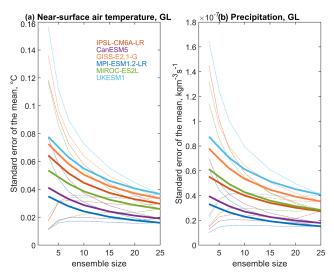
**Figure 12.** Ensemble size and spread. Standard error of the mean of anomalies calculated for different ensemble sizes across the different models for two key surface variables: global-mean near-surface air temperature (a) and global-mean precipitation (b). Shown are means (thick line) and 5–95th percentile ranges (see Sect. 2.2).
