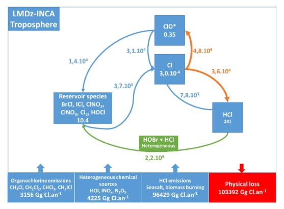
Figure 2: Simplified cycle of tropospheric Cl<sub>y</sub> species in the reference simulation. Fluxes through the reactions are in Gg Cl.yr<sup>1</sup>. Heterogeneous reactions are represented in green. The main loss pathways for atomic chlorine are in orange. The numbers in the boxes represent the mass balances of the species families in Gg Cl.
