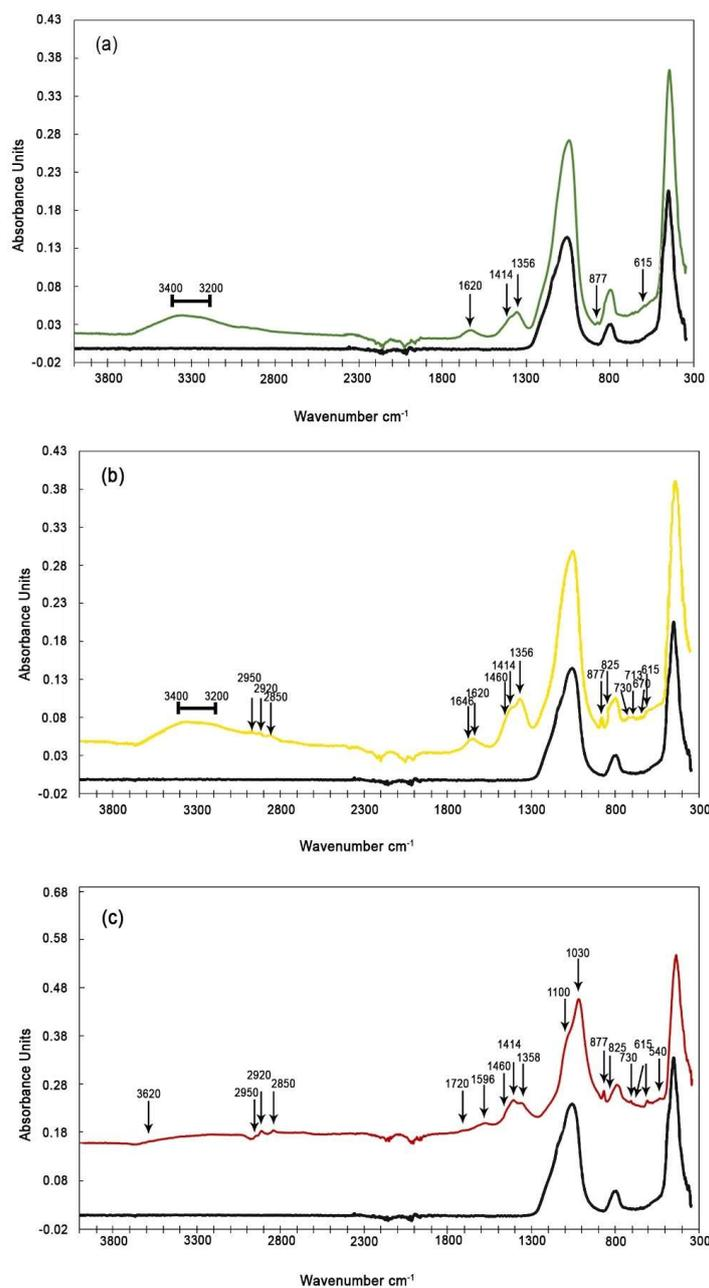
**Figure 3.** FTIR spectra of (a) suburban  $PM_{10}$  filter (BF station); (b) urban  $PM_{10}$  filter (GC station); and (c) urban  $PM_{2.5}$  filter (DB station). For each spectrum, we also report the spectrum of a blank quartz filter (black line) for comparison.
