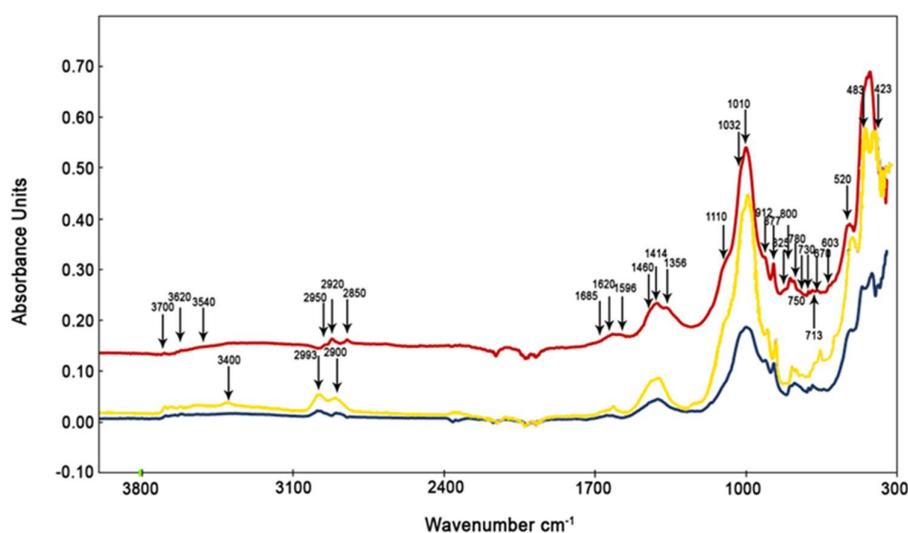
**Figure 4.** FTIR spectra of urban  $\text{PM}_{10}$  (GC, yellow line) and  $\text{PM}_{2.5}$  (DB, red line) filters. Blue line is FTIR spectrum of Saharan dust deposited in Palermo.
