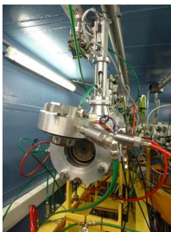
Figure 2. Targetry “hatch tip” low current (<2 \mu\text{A} ) for development.
