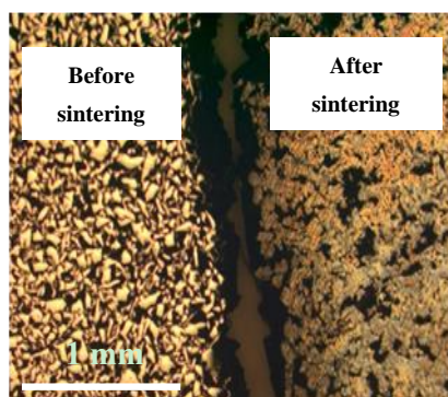
Figure 8. Micrography of polished samples before and after sintering at (800 °C).
