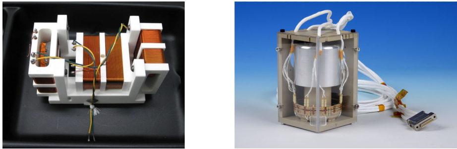
Fig. 29 MGF inboard sensor and MGF outboard sensor in protection housing: total instrument mass \tilde{0}.77 kg; power consumption \tilde{4}.4 W (images taken from Baumjohann et al. 2020)
