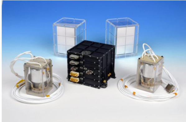
Fig. 19 MPO-MAG: Sensor flight models (left and right in front) with electronics box (black, center) and the thermal housing (in the back). Instrument mass 2.5 kg; power consumption 5.0 W (average); Image taken from Heyner et al. (2021)
