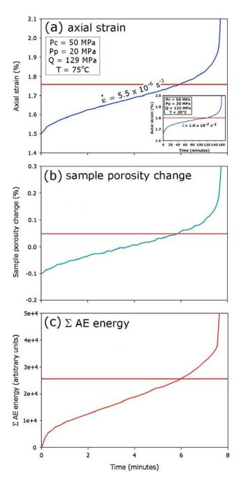
**Figure 2.** Conventional creep experiment on DDS showing the evolution over time of (a) axial strain, (b) porosity change, and (c) cumulative AE energy under a constant Q of 129 MPa. Red lines indicate the estimated positions at which the sample enters accelerating tertiary creep. Inset in Figure 2a shows a curve from an experiment at 20°C held under a similar constant stress [from *Heap et al.*, 2009].
