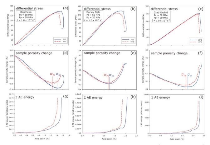
**Figure 1.** Constant strain rate experiments on samples of BHS, DDS, and COS at both  $20^{\circ}$  (solid blue lines) and  $75^{\circ}$ C (dashed red lines): (a-c) stress-strain curves, (d-f) porosity change curves, and (g-i) the output of cumulative AE energy for each of the sandstones.
