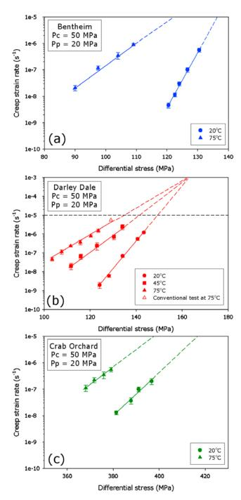
**Figure 3.** Creep strain rate data from stress-stepping creep experiments on samples of (a) BHS, (b) DDS, and (c) COS at both 20° (solid circles) and 75°C (solid triangles). Open triangle in Figure 3b represents the single conventional creep experiment on DDS (see Figure 2); data from an experiment on DDS at 45°C (see discussion) are also shown in Figure 3b.
