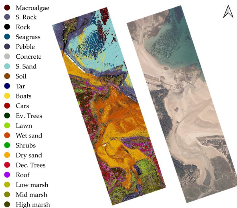
Figure A1. Projected 3D map of the habitats obtained with the predictions of a random forest classifier on green spectral features; orthoimage of the study area. The orthoimage was captured in 2014, while lidar data are not contemporaneous as they date from 2019. S. = submerged, Ev. = evergreen, Dec. = deciduous.
