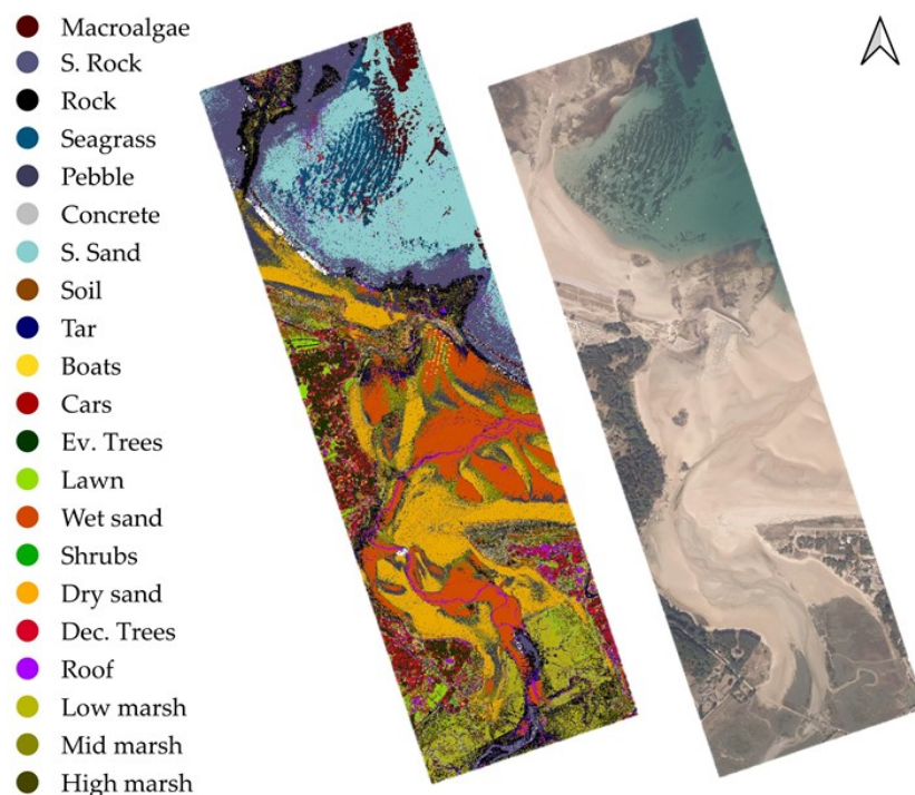
Figure A2. Projected 3D map of the habitats obtained with the predictions of a random forest classifier on green spectral features and infrared intensities; orthoimage of the study area. The orthoimage was captured in 2014, while lidar data are not contemporaneous as they date from 2019. S. = submerged, Ev. = evergreen, Dec. = deciduous.
