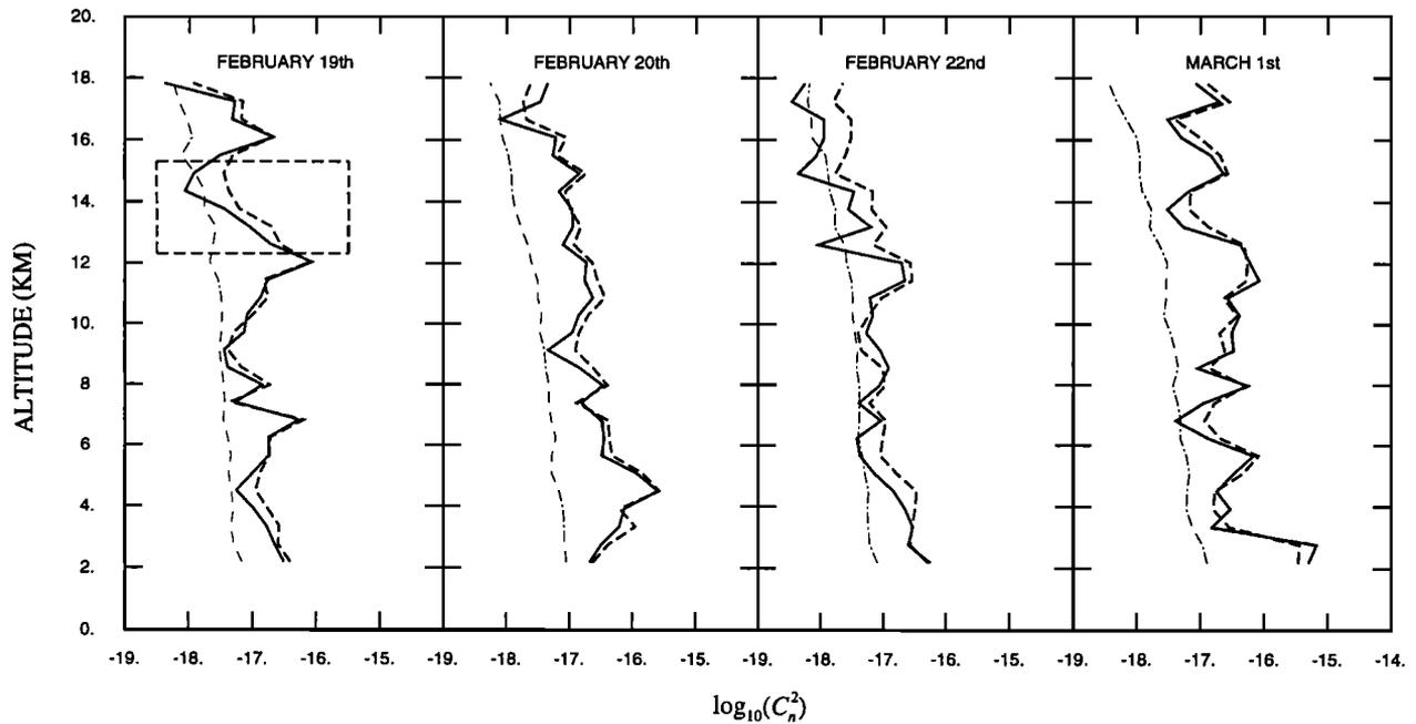
**Figure 2.** Vertical profiles, in logarithmic scales, of estimated  $C_n^2$  deduced from the spectral and horizontal variance methods shown by dashed and solid lines respectively during the four balloon data sets at the radar range resolution (600 m). The noise level of the reconstructions is shown by a dash-dotted line. The humidity contribution is not introduced in the estimations. The dashed region is shown in Figure 1.
