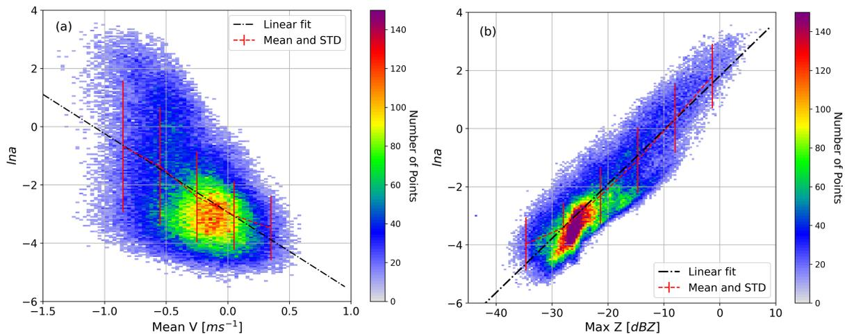
**Figure 14.** Correlation of (a) Mean velocity versus  $lna$  and (b) Maximum reflectivity versus  $lna$  for cloud profiles, where color bar indicates the number of profiles
