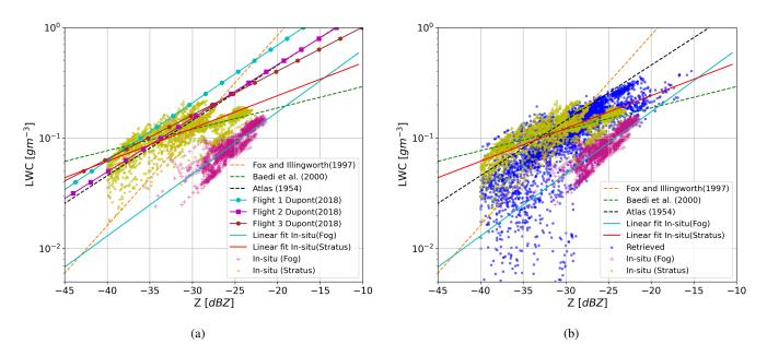
**Figure 10.** Comparison of in-situ LWC and radar reflectivity relation with (a) available literature for fog and clouds, (b) retrieved LWC and BASTA radar reflectivity relation.
