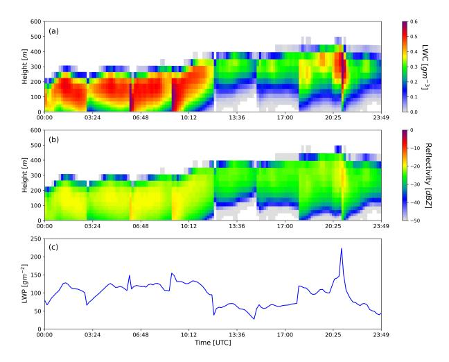
Figure 4. Simulations from AROME model for 16 November 2018 showing (a) True LWC in  $gm^{-3}$ , (b) Synthetic reflectivity and (c) LWP.
