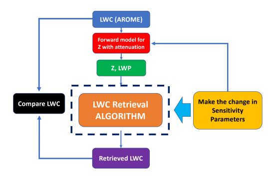
Figure 3. Flow chart for sensitivity analysis of retrieval algorithm.
