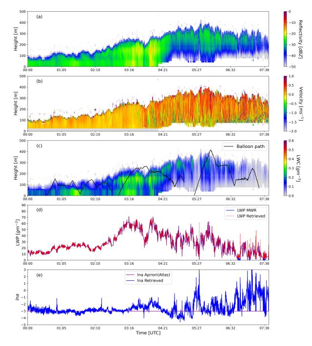
**Figure 7.** (a) Radar reflectivity Z (b) Vertical velocity (c) Retrieved LWC, (d) LWP and (e) Retrieved *lna* for 09 February 2020 case at SOFOG-3D super-site. Tethered balloon trajectory over retrieved LWC is shown in black line.
