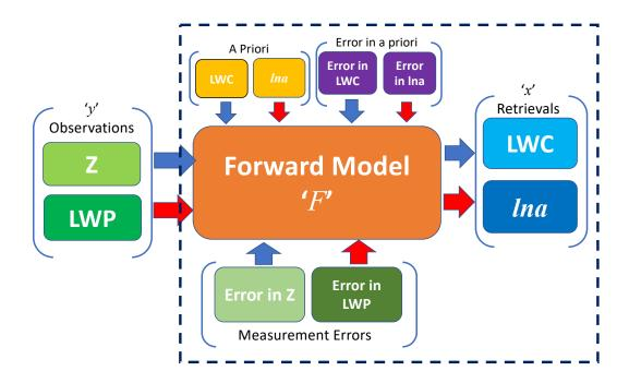
Figure 1. Schematic of LWC retrieval algorithm.
