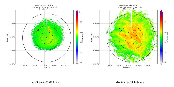
Figure 9. Scans of BASTA-mini collected for fog at  $4^{\circ}$  elevation angle. The vertically pointing radar shown as blue dot was located 1 km away from the scanning radar and cross represents the location of balloon.
