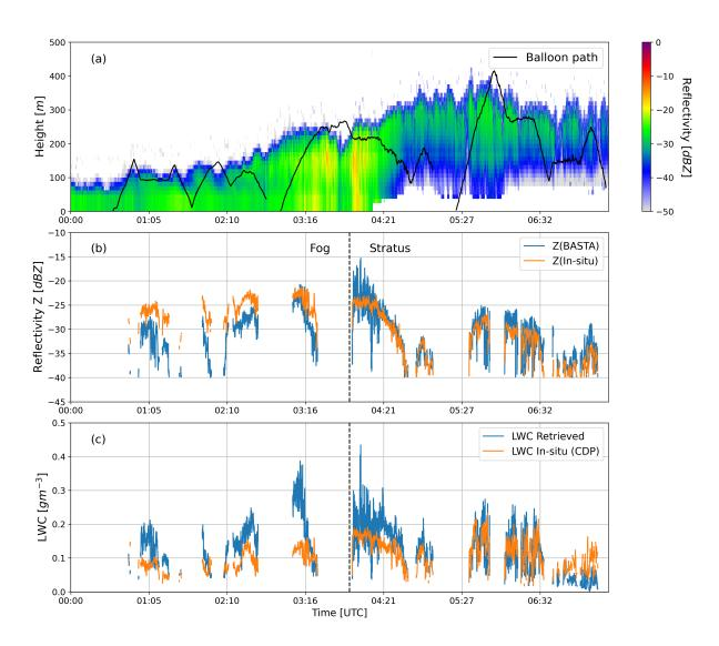
Figure 8. (a) Radar reflectivity and balloon path (b) Comparison of radar reflectivity with reflectivity calculated from CDP using DSD (c) Comparison of retrieved LWC with in-situ LWC
