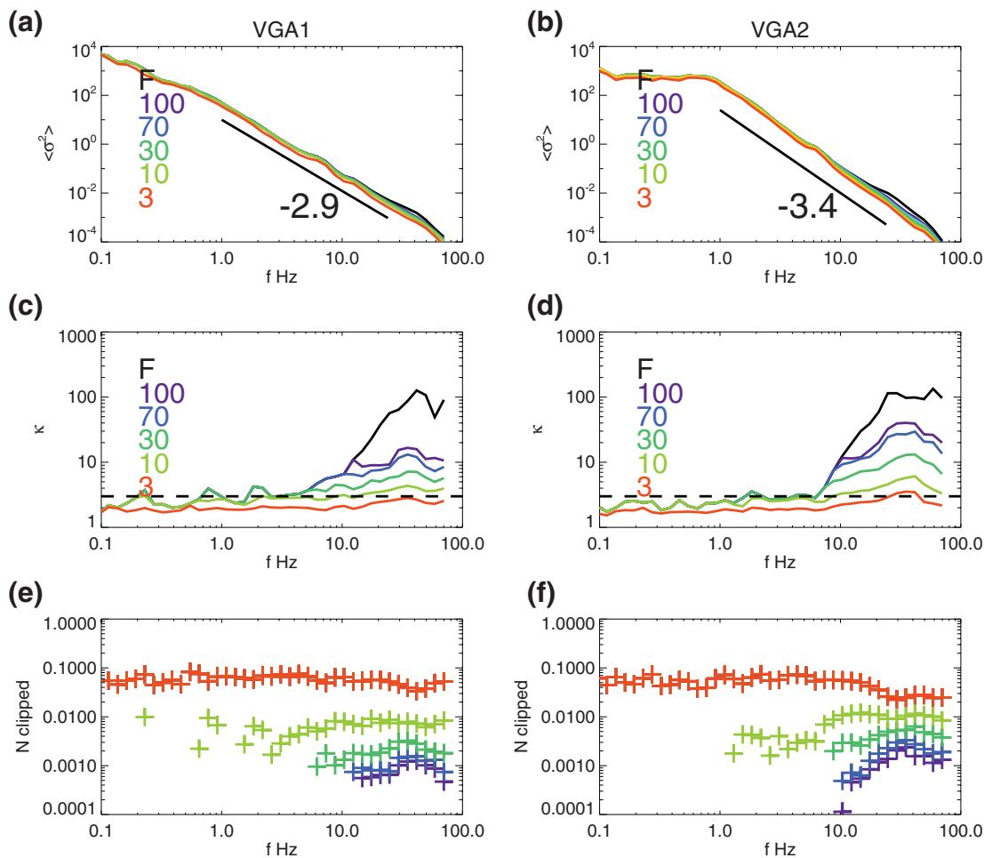
**Figure 4.** (a and b) CWT spectra  $\langle \sigma_s^2 \rangle$  for VGA1 and VGA2 (black); colors correspond to conditioned spectra. (c and d) Effect of conditioning on wavelet kurtosis for VGA1 and VGA2. (e and f) Percentage of clipped wavelet coefficients at each conditioning level. CWT, continuous wavelet transform; VGA, Venus gravity assists.
