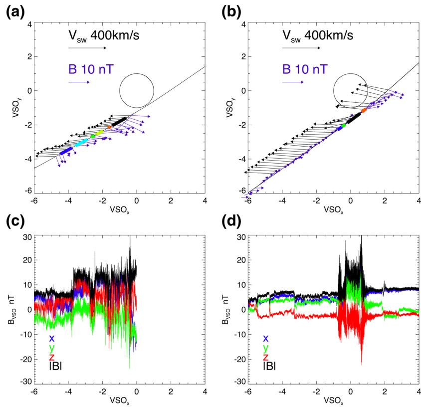
**Figure 1.** (a and b) Trajectory of PSP during VGA1 and VGA2 in VSO  $x$  -  $y$  plane. Black arrows show scaled plasma flow; purple arrows show measured magnetic field. (c and d) Vector magnetometer measurements for VGA1 and VGA2 ( $x$ ,  $y$ ,  $z$ /blue, green, red) with the magnitude (black). PSP, Parker Solar Probe; VGA, Venus gravity assists.
