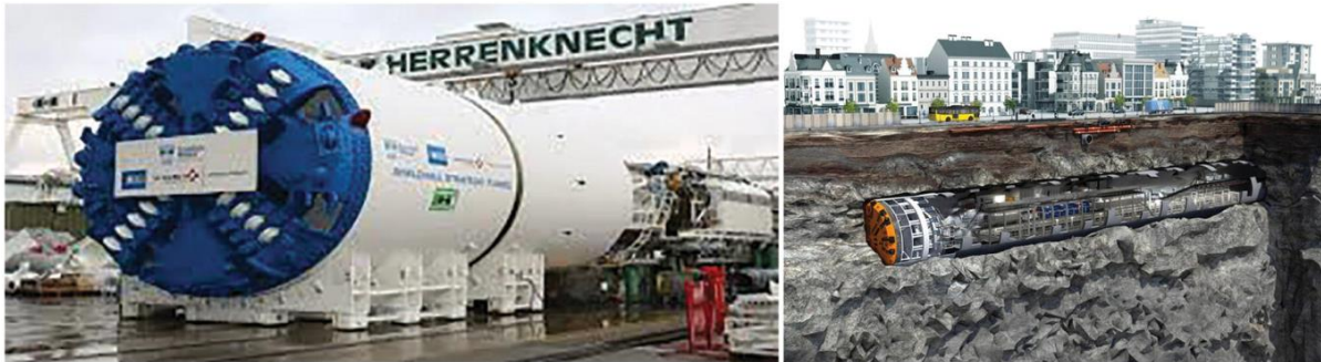
Figure 17.14 (Left) Picture of a Tunnel-boring Machine (TBM) of the Herrenknecht company, one of the world's leader in the field during its construction phase (Source: ©Scottish Plant, https://www.scottishplant.co.uk/heres-a-boring-story/ ). (Right) Artistic view of a TBM while digging an urban tunnel (Source: ©Medium.com https://medium.com/netive-in/17th-tunnel-boring-machine-lowered-for-metro-iii-tunnel-work-1c5f7360af29 ).
