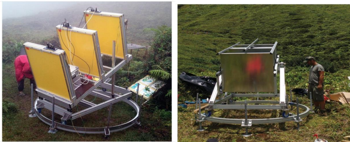
Figure 17.1 Two versions of muon telescopes operating on the Soufrière of Guadeloupe (Rocher Fendu location). The electrical power is provided by solar panels and a Wi-Fi link allows daily data download and software parameterization. The mechanical frames allow zenith/azimuth orientations
