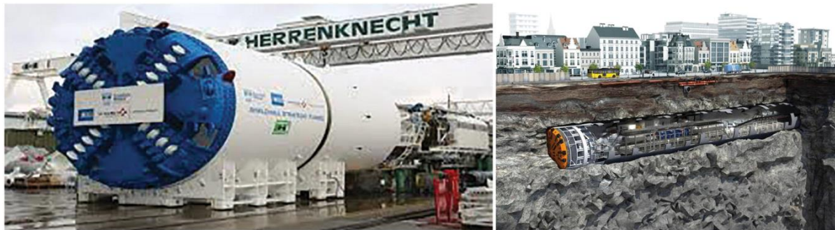
Figure 17.14 (Left) Picture of a Tunnel-boring Machine (TBM) of the Herrenknecht company, one of the world's leader in the field during its construction phase
