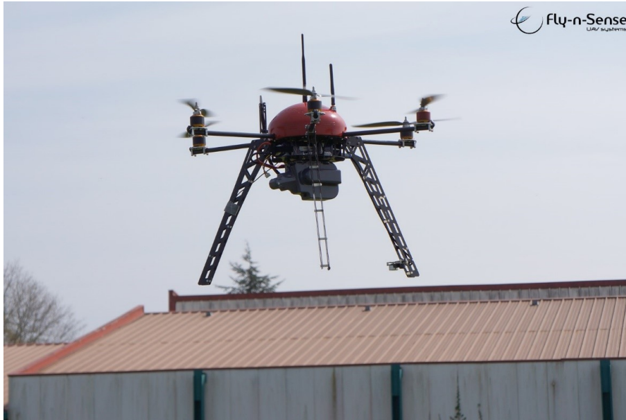
Figure 2. LOAC on board an unmanned aerial vehicle of the Fly N Sense Company (LOAC is on the black box at the bottom of the vehicle).
