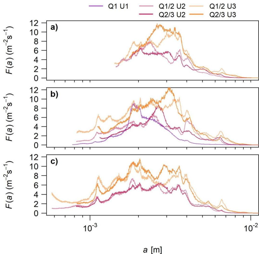
**Figure 3.** Average frequency distribution of the bubble number flux ( $F$ ) per bubble radius ( $a$ ) for the different experimental runs in flume F1 (**a**), flume F2 (**b**) and flume F3 (**c**) for different bubble flux levels ( $U$ ) and discharge levels  $Q$  ( $Q1$  and  $Q2$  in flumes F1 and F2;  $Q2$  and  $Q3$  in flume F3).
