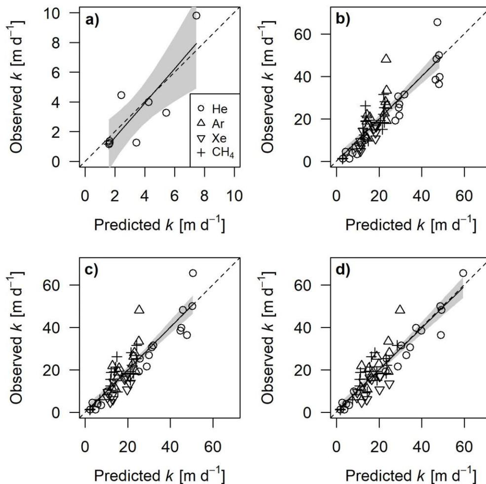
**Figure 5.** Observed vs. predicted gas exchange velocity ( $k$ ) for the models LS70 (a), W97 (b), W93m (c), W93w (d). The dashed line is the 1:1 line. The solid line is the linear regression. For regression equations, see Table S1. The grey shading denotes 95% confidence intervals of the regression line. None of the regression intercepts is significantly different from 0 and none of the slopes is significantly different from 1.
