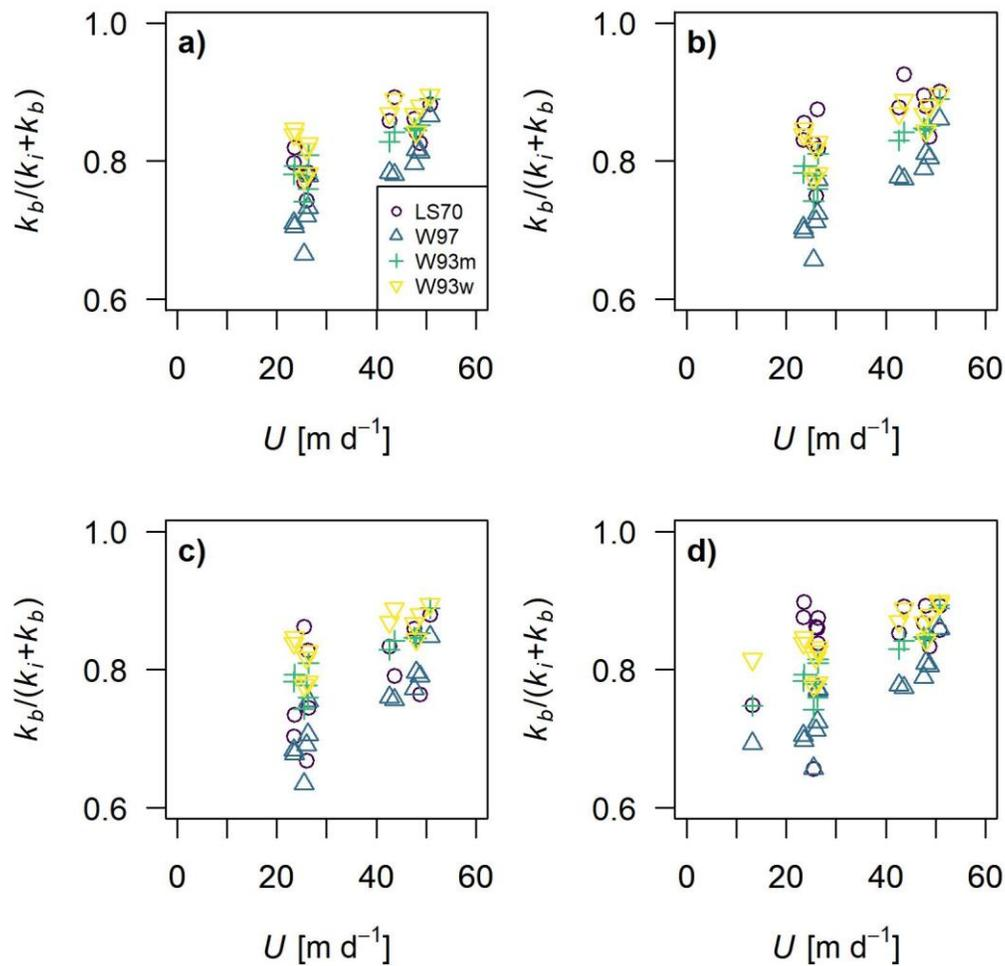
**Figure 6.** Relative contribution of bubble-mediated to total gas exchange velocity ( $k_b/(k_i+k_b)$ ) according to the models LS70, W97, W93m, and W93w, for Helium (a), Argon (b), Xenon (c), and Methane (d) for experiments with bubble injections. Shown are bootstrap median values. The 95% confidence intervals around these medians are (-0.06, +0.11) (LS70), (-0.13, +0.11) (W97), (-0.12, +0.10) (W93m), and (-0.11, +0.08) (W93w) as medians across all observations.
