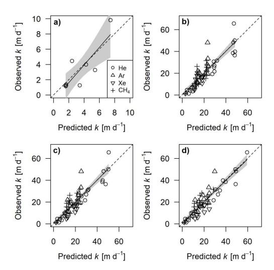
**Figure 5.** Observed vs. predicted gas exchange velocity (k) for the models LS70  $(\mathbf{a})$ , W97  $(\mathbf{b})$ , W93m  $(\mathbf{c})$ , W93w  $(\mathbf{d})$ . The dashed line is the 1:1 line. The solid line is the linear regression. For regression equations, see Table S1. The grey shading denotes 95% confidence intervals of the regression line. None of the regression intercepts is significantly different from 0 and none of the slopes is significantly different from 1.
