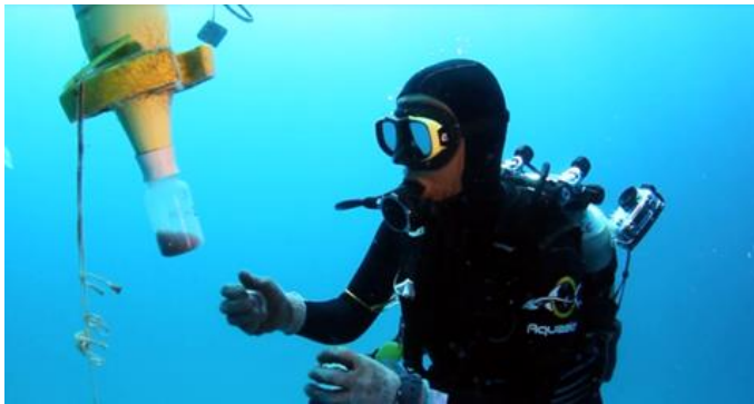
Figure 1. (a) Mesocosms ( \sim 50 \text{ m}^3 ) deployed in the framework of the VAHINE project. (b) Sediment traps screwed onto the base of the mesocosms and were sampled daily by SCUBA divers.
