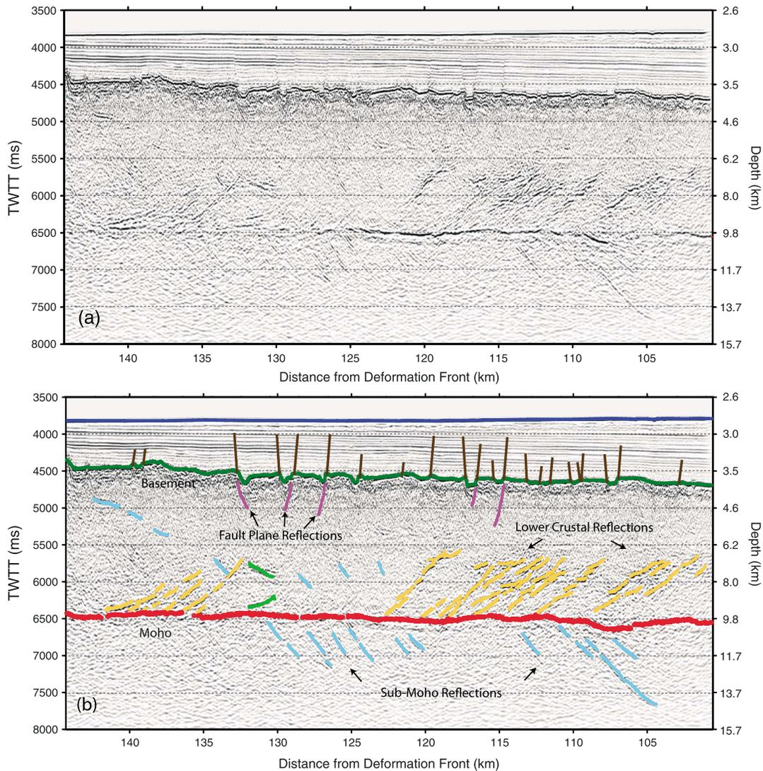
**Figure 5.** MCS (a) image and (b) interpretation of the portion of the Oregon transect with lower crustal ridgeward dipping reflections. Right-hand side labels are the approximate depths corresponding to the two-way traveltimes on the left-hand side.
