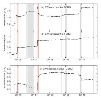
**Figure 6.** East-west daily averaged displacement recorded between 2005 and 2011 by the (a) DERG and (b) the FERG station; displacement is positive eastward; (c) E-W FERG-DERG baseline length; lengthening is positive. Shaded areas indicate eruptive periods (summit/proximal eruptions (grey); distal eruptions (red)).
