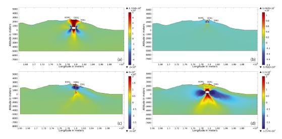
**Figure 14.** Horizontal stress change (color, in Pa) as a function of the longitude and altitude, for the various loading cases of the eruptive cycle presented in Figure 13. Stress is positive in tension, and negative in compression. Tension in the summit edifice, due respectively to (a) the summit inflation and (d) the eastward displacement of the eastern flank. (b) Compression in the summit edifice and (c) loading of the eastern flank. Parameters of the models are similar to Figure 13.
