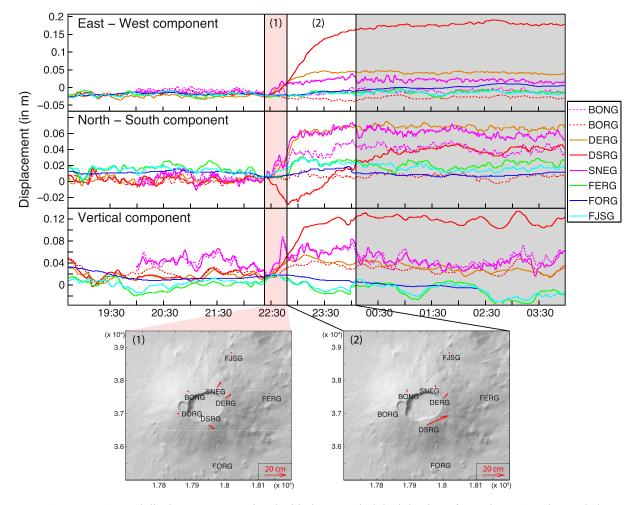
**Figure 5.** Ground displacements associated with the summit dyke injection of 20 July 2006 and recorded by the OVPF GPS stations. Labeled vertical solid lines correspond to the characteristic times presented in the results. Map sketches indicate the displacement vectors corresponding to each GPS station. Shaded grey areas indicate eruptive periods.
