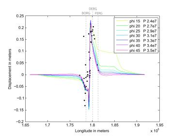
**Figure 12.** Interdistal mean horizontal displacements (same as Figure 11) and theoretical displacements computed for various values of  $\phi$ , for the model described in section 4.1.3. In each case, dyke overpressure is adapted to get the observed displacements at the dyke boundaries, whereas  $\phi$  controls the displacement at the base of the summit cone (westernmost and easternmost values). Low  $\phi$  values do not allow to fit the observed displacement at FERG.
