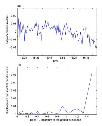
**Figure 4.** (a) One hour record of the FERG GPS vertical component noise measured before the 30 March 2007, strong displacement preceding the eruption. (b) Periodogram computed for the 1 h noise sample presented in Figure 4a.
