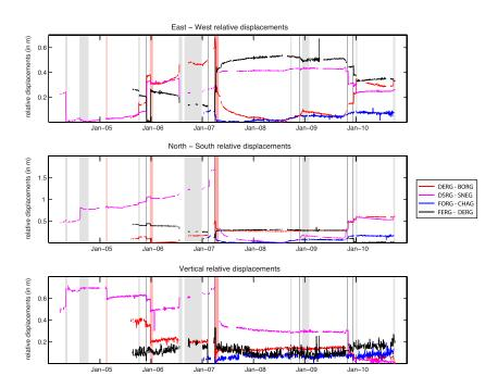
**Figure 7.** Baseline changes recorded for four station pairs between 2004 and 2010. Shaded areas indicate eruptive periods (summit/proximal eruptions (grey); distal eruptions (red); see Table 1 for details). Distance samples are daily averages.
