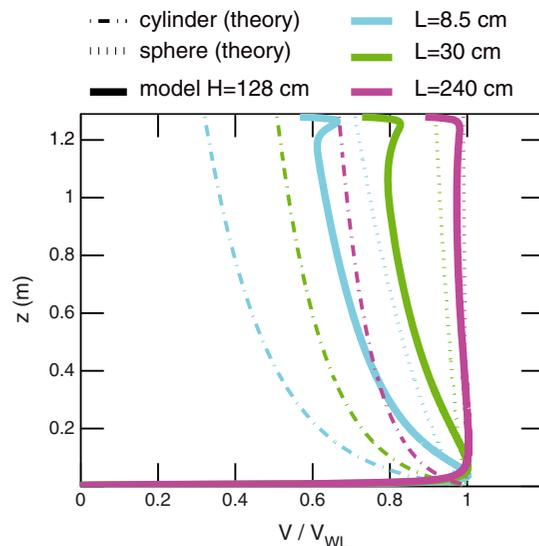
**Figure 15.** Comparison between  $V/V_{WL}$  observed in the open boundary simulations (solid lines) and the drag reduction predicted for a sphere (short dash lines [*Happel and Brenner*, 1973, pp. 318]) or for a cylinder (dot-dashed lines [*Happel and Brenner*, 1973, pp. 342]) for  $H=128$  cm.
