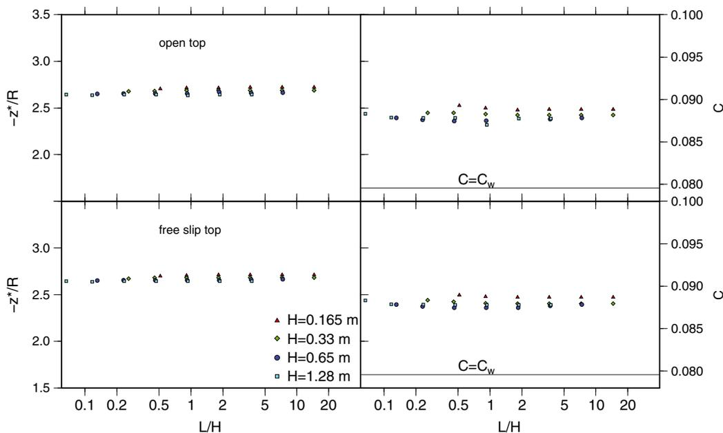
**Figure A1.** The parameters  $z^*$  (left) and  $C$  (right) as determined from the centerline temperature profile by a nonlinear fit to equation 9. While the size of the box and the choice of top boundary conditions have a significant effect on the velocity, the temperature in the plume is principally insensitive to these geometrical considerations.
