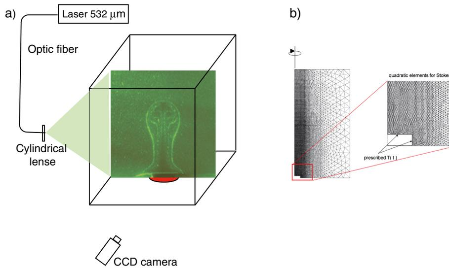
**Figure 2.** Experimental set-up: (a) laboratory experiments and (b) mesh used for the axisymmetric numerical simulations. The numerical resolution is finest around the heater with an average nodal point spacing of 0.2 mm.
