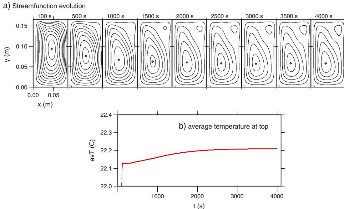
**Figure 12.** (a) Evolution until  $t = 4000$  s of the streamfunction (a) in the smallest box ( $H = 16.5$  cm,  $L = 8.5$  cm). After an initial apparent steady state with symmetrical streamfunction the pattern becomes asymmetric. (b) average temperature in a rectangle in the top left corner of 5 mm wide by 2 mm high.
