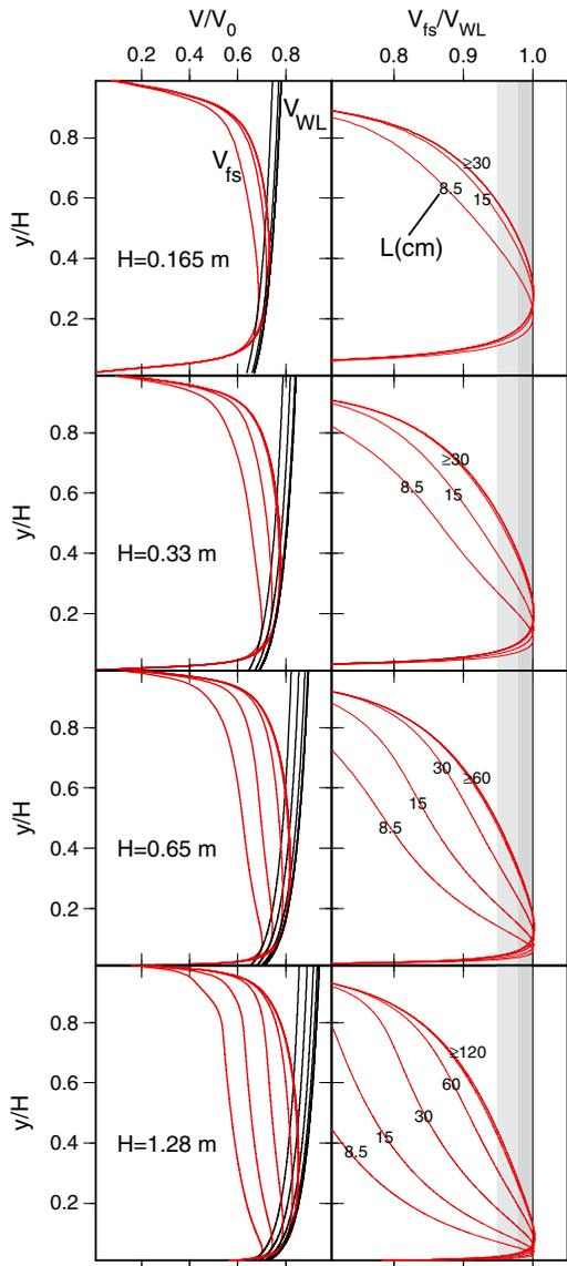
**Figure 9.** Comparison of modeled axial velocity  $V$  and prediction  $V_{WL}$  for variable  $H$  and  $L$ . In the left column we plot  $V/V_0$  in red and  $V_{WL}/V_0$  in black. The ratio  $V/V_{WL}$  is shown in red in the right column. The light grey band indicates where this ratio is  $>0.95$ . The dark grey band shows where this ratio is  $>0.98$ . The small numbers on the curves show the width of the box  $L$  (in cm).
