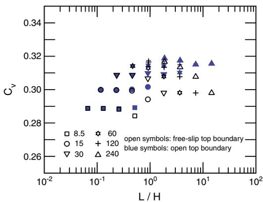
**Figure A3.** Constant  $C_v$  in the velocity scaling (10) determined for the free slip (black symbols) and the open boundary (blue symbols) cases. Domain width  $L$  is indicated (in cm) in the legend for the different symbols.
