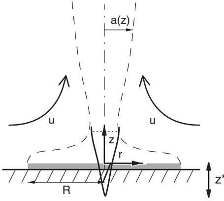
**Figure 1.** Modified from *Whittaker and Lister* [2006b]. Sketch of the steady state geometry of a plume rising from a disk heater of radius  $R$ . Above a certain height the temperature distribution in the plume is similar to that of a plume rising of a point heater at virtual depth  $z^*$ .
