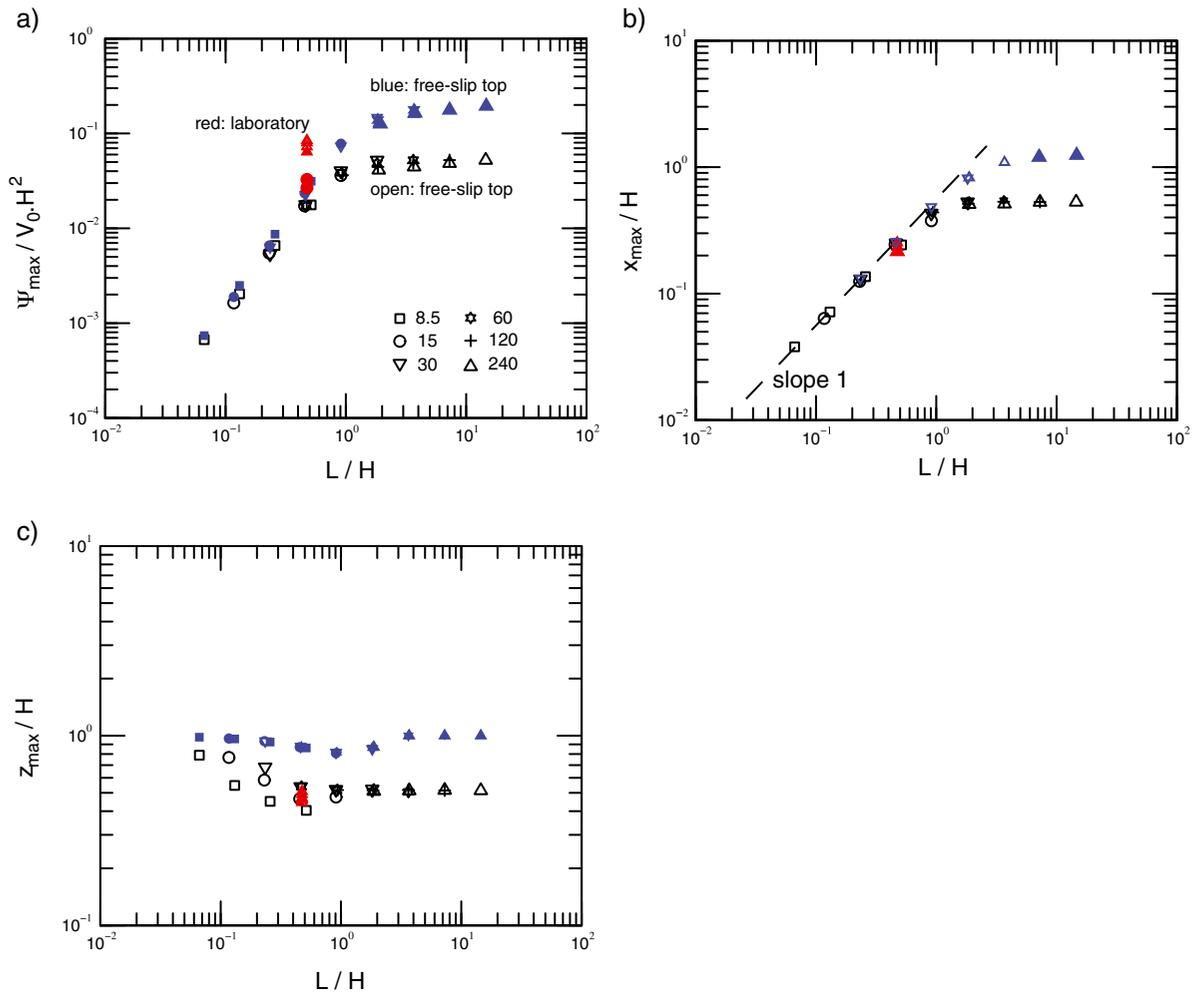
**Figure A5.** Characteristics of the stream function maximum as a function of the domain aspect ratio. In black, the numerical experiments with a free surface, in blue the ones with the top open boundary, in red the laboratory experiments for temperature differences between 21 and 54°C. Symbols indicate the width of the models (indicated in cm in the legend in frame a). a) non-dimensional streamfunction maximum, b) non-dimensional horizontal position of maximum, c) non-dimensional height.
