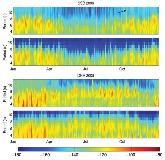
**Figure 10.** Real and synthetic noise power spectra variations for stations in France (SSB) and in a small island close to Antarctica (DRV). For each station, real (top panel) and synthetic (bottom panel) daily spectra are plotted in dB with respect to acceleration (colour) for the years 2008 and the period band 3–10 s The noise peak designed by the arrow corresponds to the source shown on Fig. 11.
