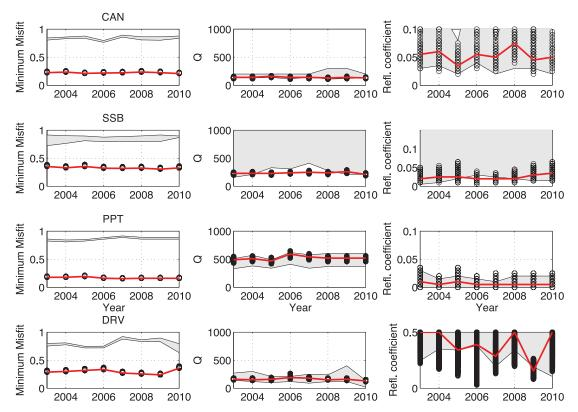
**Figure 8.** For years 2003 to 2010, the lowest mistfit (left-hand side) and the corresponding attenuation (middle) and reflection coefficient (right-hand side) are plotted in red. Circles correspond to all the misfit values within 5 per cent of the minimum value (left-hand side) and the corresponding Q (middle) and  $R^2$  (right-hand side). The grey areas correspond to the highest correlation values (left-hand side) and the corresponding values for Q (middle) and  $R^2$  (right-hand side).
