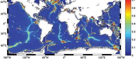
Amplification factor for the seismic wave period T=10s
