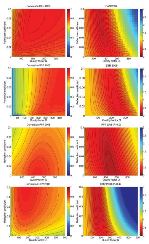
Figure 5. Correlation (left-hand side) and misfit ( $L_1$  norm, right) between real and synthetic spectra as a function of seismic attenuation and ocean wave coastal reflection coefficient for for two continental stations, CAN in Australia and SSB in France and an island station PPT in french Polinesia (Tahiti).
