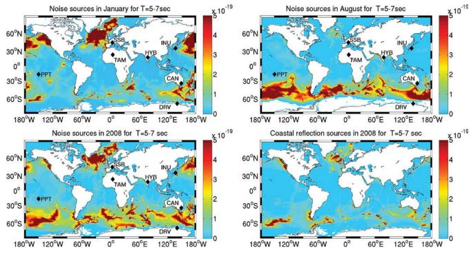
Figure 3. Noise source locations in 2008 for the period band 5–7 s in January (upper left), in August (upper right), averaged over the year (lower left), for sources generated by coastal reflection only (lower right).
