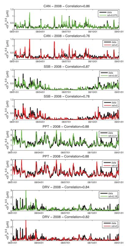
Figure 7. Real (black) and synthetic (colour) power spectra variations over year in displacement (m) for two continental stations, CAN in Australia and SSB in France, an island station PPT in french Polynesia (Tahiti) and a station in Antarctica DRV. Synthetic spectra are computed with (green) and without (red) taking into account ocean wave coastal reflection.
