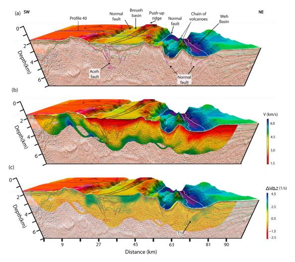
**Figure 8.** (a) Three-dimensional perspective view of the profile WG2 with bathymetry. The chain of volcanoes is prominent here and several normal faults are shown. Location of profile-40 is also marked. (b) Same as Figure 8a with inverted velocity model superimposed. (c) Same as Figure 8a with the velocity gradient superimposed. The interpreted fault is aligned with the velocity gradient plot marked below the Weh Basin. T1: marks the coincident velocity gradient and the normal fault.
