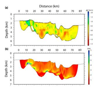
**Figure 4.** (a) Velocity anomaly: The difference between the OBS tomography derived 2D starting model and the final inversion result. (b) The derivative weight sum (DWS) for the best fit model. The DWS is calculated adding the elements of each column of the Frechet derivative matrix. It is a dimensionless measure of the sensitivity of the data to a model parameter [van Avendonk et al., 1998]. The DWS is plotted in between 0.1 and 7.
