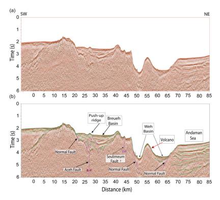
**Figure 5.** Time migrated seismic image along the profile WG-2: (a) uninterpreted and (b) interpreted. V.E. is 4:1 (at water velocity 1.5 km/sec). The data was processed using a standard processing technique [*Chauhan et al.*, 2009].
