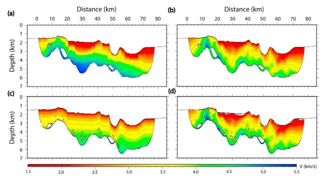
**Figure 3.** Travel time inversion conducted using two different starting models. (a) The 2D starting model based on OBS tomographic results [*Chauhan et al.*, 2009] and (b) the final inversion result. (c) Starting model obtained by hanging a 1D average velocity profile on the seafloor and (d) corresponding final inversion result.
