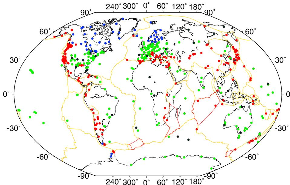
**Figure 1.** ITRF2008 sites with time-span longer than three years. Red: sites close to plate boundaries or in deformation zones. Blue: sites located in GIA regions. Black: sites with normalized velocity residuals larger than 3, or raw residuals larger than 3 mm/a. Green: our final selection of 206 sites. *Bird's* [2003] plate boundaries are shown in orange, and the four additional MORVEL plates in red [DeMets *et al.*, 2010].
