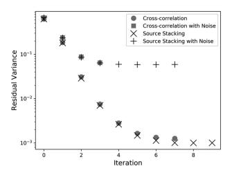
**Figure 6.** The evolution of variance reduction as a function of iteration for each of the experiments performed. Note that for iteration 1 with noise, the residual variances for source-stacking inversion and when the additional cross-correlation step is included, plot on top of each other.
