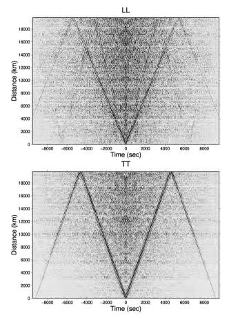
**Figure 3.** Stacked L–L (top panel) and T–T (bottom panel) crosscorrelations between station pairs for the entire synthetic data set. The strongest energy corresponds to group velocities of  $3.75 \text{ km s}^{-1}$  for L–L and  $4.35 \text{ km s}^{-1}$  for T–T, which are in the middle range of group velocities for fundamental mode Rayleigh and Love waves, respectively.
