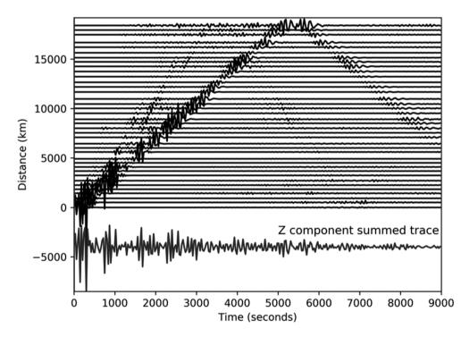
Figure 2. An example of vertical component 10 000-s long traces calculated at station TATO in the 1-D average model derived from SEMUCB-WM1 (French & Romanowicz 2014). 38 different events are shown here, aligned on origin time and ordered as a function of epicentral distance. The frequency band of the calculation is 400–60 s. The bottom trace is the sum of the 38 aligned traces.
