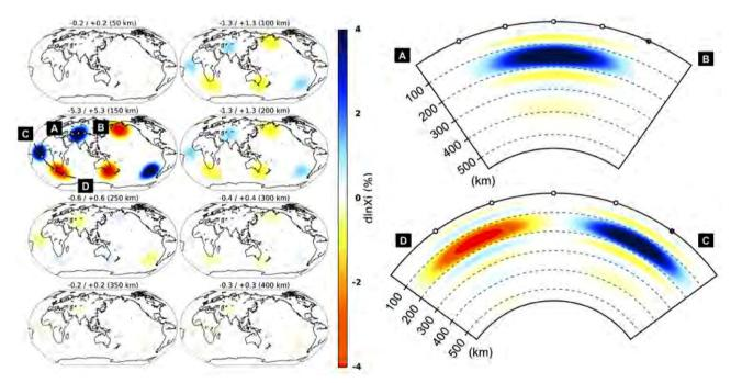
Figure 5. Anisotropic parameter  $\xi$  variations in the 'BLOB' model, plotted in map view at several depth (left-hand panel), in percent relative to the global mean (isotropic) at that depth. Extrema of each map are shown above the corresponding map. Right-hand panels present depth cross-sections along two profiles A - B and C - D as indicated on the 150 km map.
