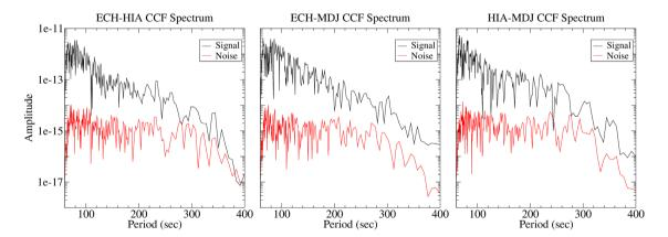
Figure 12. Comparison of the spectra of the cross-correlations traces shown in Fig. 11. The traces have been filtered with corner frequencies of 20 and 800 s. Note the logarithmic scale on the *y*-axis.
