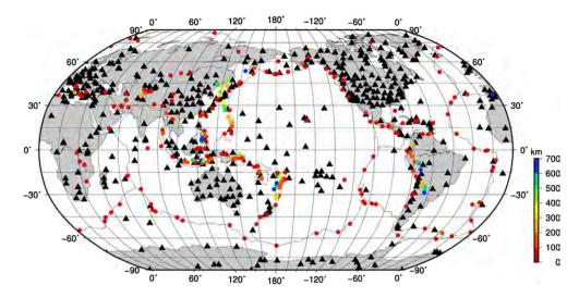
Figure 1. The distribution of events and stations used for the synthetic experiments presented in this paper. It consists of the 273 earthquake sources and 537 stations used for the development of global mantle model SEMUCB-WM1. The colours indicate the depths of sources.
