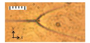
FIG. 8. Solitary PFCD in a 20- $\mu$ m-thick N<sub>TB</sub> layer of CB7CB in a planar cell. Scale:  $2 \mu m$  each small div. Polarizer along x.
