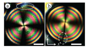
FIG. 1. Imperfect toric focal conic formations in the  $N_{\text{TB}}$  phase of a 20- $\mu$ m-thick CB7CB layer in a 90°-twist cell. (a) 8.1 V, 10 kHz and (b) after switch off from 15 V, 1 kHz. Defect regions are encircled. The appearance of these defects is a first step in the transformation of TFCDs into PFCDs. Notice the small grainy defects all along circles. Crossed polarizers with their axes along (*x*, *y*). Scale bar: 10  $\mu$ m.
