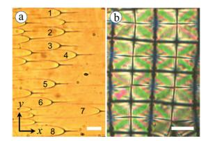
FIG. 2. Focal conics in the  $N_{\rm TB}$  phase of CB7CB, close to its setting point: (a) PFCDs and FCDs (see later for eccentricities of the numbered conics here), (b) electrically generated (8 V, 1 kHz) PFCDs, arranged along the substrate rubbing direction. The precursor *N* was: (a) aligned along *x*, (b) homeotropic. Single polarizer along *x* in (a), crossed polarizers along *x* and *y* in (b). Scale bar: 20  $\mu$ m.
