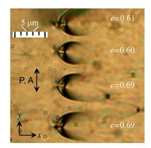
FIG. 7. Quasiparallel FCDs in a 20- $\mu$ m-thick layer of CB7CB in a planar cell at  $0.6^{\circ}$ C below the setting point and subjected to a 30 V, 1 kHz field. The FCD ellipses are connected by a set of attached quantized dislocations approximately parallel to the minor axes. P and A denote polarizer and analyzer.
