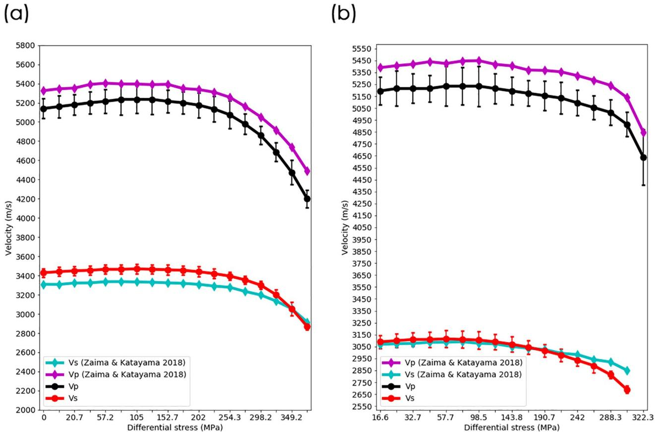
**Figure 8.** Evolution of  $V_p$  and  $V_s$  of (a) dry and (b) wet data. The black and red circle represent the numerical simulated best-fit results of  $V_p$  and  $V_s$ , respectively. The diamond shapes are the results from Zaima and Katayama (2018), which are calculated from the hand-picked first arrivals.
