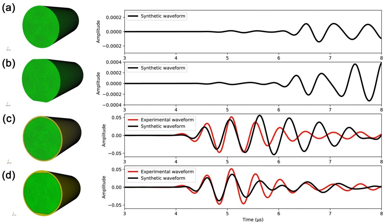
**Figure A1.** The four models tested in this study and their synthetic waveform (a) cylindrical model with free-boundary, (b) side-cut cylindrical model with free-boundary, (c) cylindrical model with surrounding silicone jacketing model and (d) side-cut cylindrical model with surrounding silicone jacketing model.
