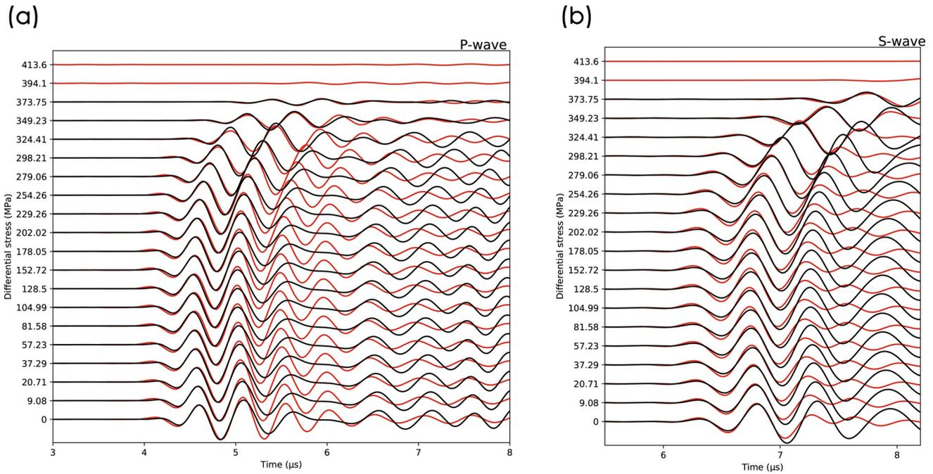
**Figure 11.** The result of (a) P- and (b) S-wave strain waveform fitting of dry data using Equation 3 to find the best-match model with proper  $V_p$ ,  $V_s$ ,  $Q_p$ ,  $Q_s$ . The black lines are the best-match synthetic waveforms. The red lines are the experimental data. The y-axis indicate the deformation progress and correspond to a condition of  $\Delta\sigma$ . The x-axis represents the time of wave propagation.
