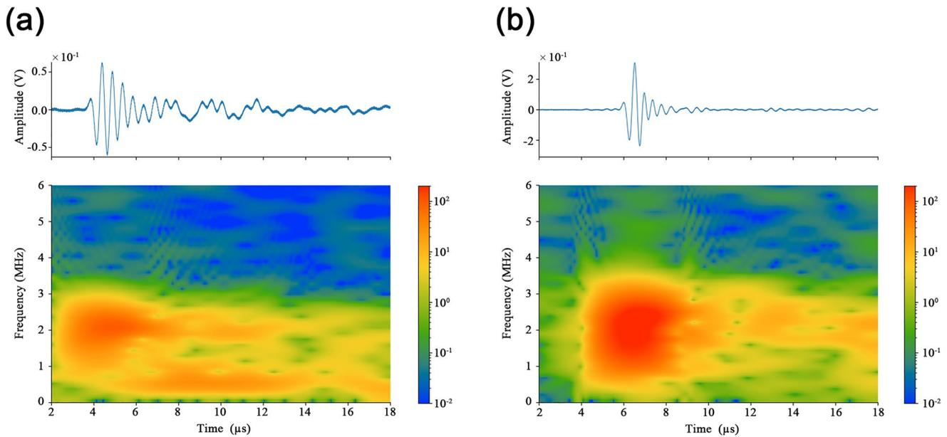
**Figure 3.** The (a) P- and (b) S-wave spectrogram of experimental data for 0 MPa differential stress.
