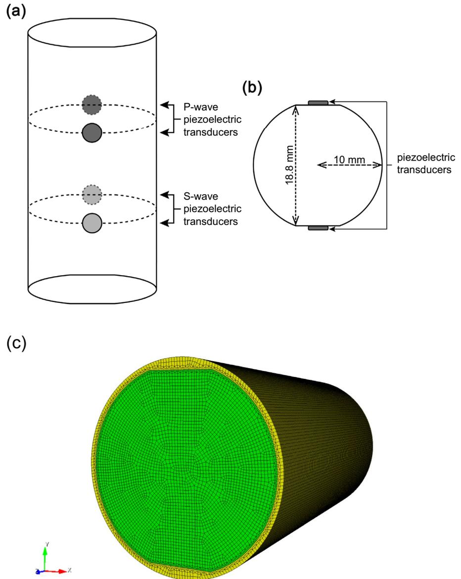
**Figure 1.** The schematic diagram of the geometry of sample, the position of the transducers and the numerical model used in this study. (a) The general view of the experimental setting of the sample. (b) The cross-section of the sample. (c) The distorted hexahedral mesh of the model for spectral element method. The green region is the rock model. The yellow part represents the surrounding low-velocity material. The mesh size is approximately 0.3 mm.
