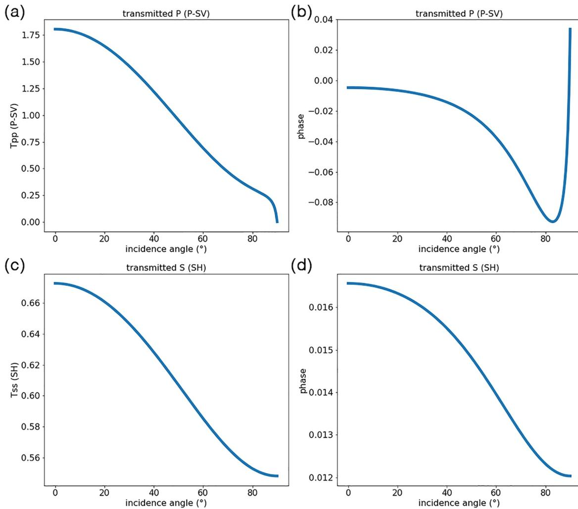
**Figure A2.** The transmission coefficient P to P (P-SV) and S to S (SH) of solid-solid surface between the granite and the silicone rubber plotted with incidence angle. The frequency range is set to the dominant frequency 2 MHz. (a) P to P (P-SV) amplitude, (b) P to P (P-SV) phase, (c) S to S (SH) amplitude, (d) S to S (SH) phase.
