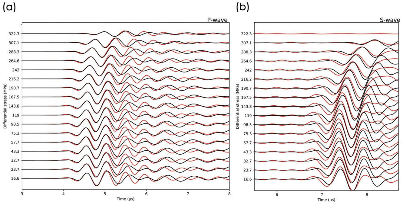
**Figure 12.** The result of (a) P- and (b) S-wave strain waveform fitting of wet data using Equation 3 to find the best-match model with proper  $V_p$ ,  $V_s$ ,  $Q_p$ ,  $Q_s$ . The black lines are the best-match synthetic waveforms. The red lines are the experimental data. The y-axis indicate the deformation progress and correspond to a condition of  $\Delta\sigma$ . The x-axis represents the time of wave propagation.
