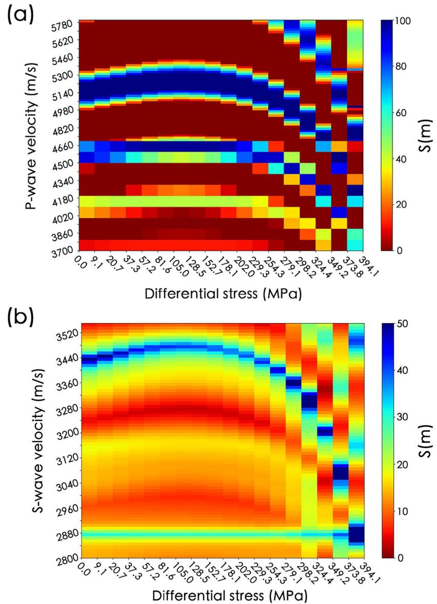
**Figure 7.** The result of waveform fitting using objective function (Equation 3). The possible trend of change in (a) P-wave and (b) S-wave velocity with increasing differential stress is shown as the high extreme of the scale (dark blue).
