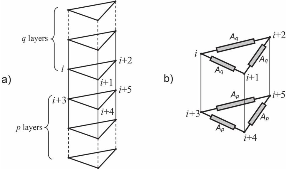
**Figure 5.** (a) Inner part of an  $m \times 3$  cylinder or globe network. (b) Equivalent diagram of the network made by the internal nodes  $i$ ,  $i + 1$ ,  $i + 2$ ,  $i + 3$ ,  $i + 4$  and  $i + 5$ .
