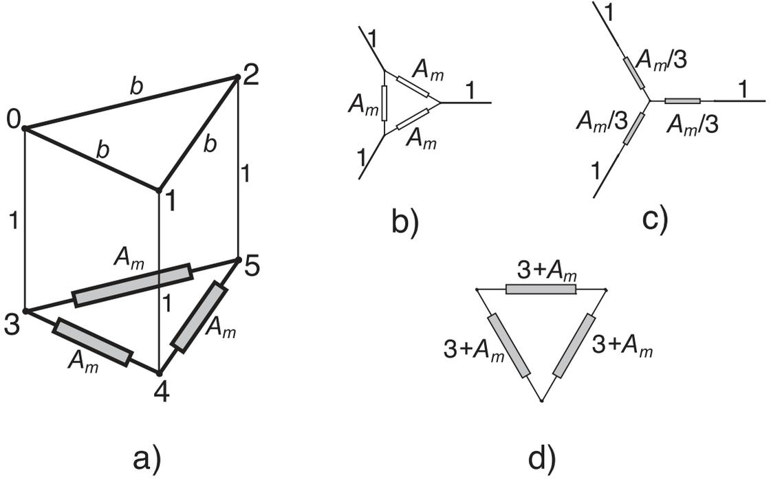
**Figure 3.** (a) Equivalent diagram of the top six nodes of the  $m \times 3$  cylinder network. (b) Diagram showing the circuit below nodes 0, 1 and 2 in figure 3(a). (c) After application of the  $\Delta$  to Y transform in the central part of figure 3(b). (d) After application of the Y to  $\Delta$  transform to the Y circuit of figure 3(c).
