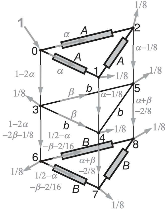
**Figure 6.** Equivalent diagram of an internal part of an  $m \times 3$  cylinder or globe network, displaying nine nodes and one intermediate frame layer.
