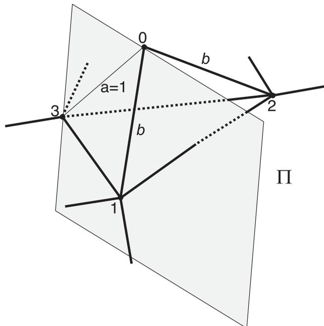
**Figure A1.** General case of a corner node 0 with three legs in a network with a plane of symmetry  $\Pi$  containing node 0 and one leg.
