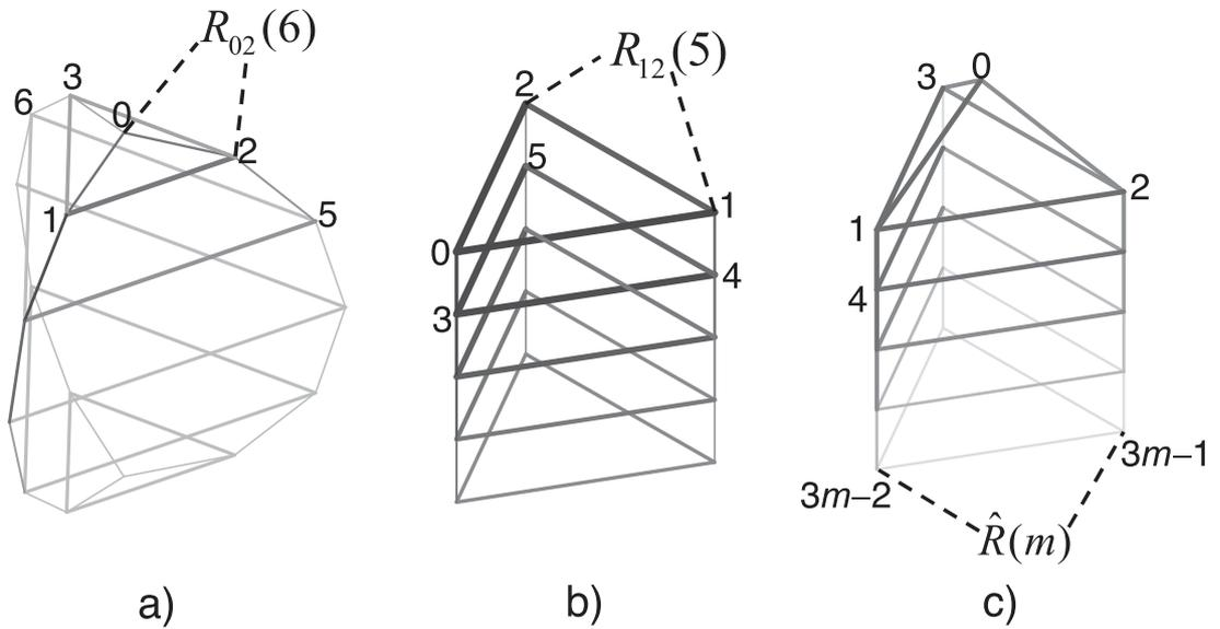
**Figure 1.** (a)  $6 \times 3$  globe network (five triangular frames perpendicular to the three-fold axis). (b)  $5 \times 3$  scaffolding or cylinder network (five triangular frames perpendicular to the three-fold axis). (c)  $5 \times 3$  tower network ( $5 \times 3$  scaffolding with a top node). The frames perpendicular to the three-fold axis are all equal to  $b$ , and all resistors linking the frames or linking the top and bottom to polar nodes, when present, are equal to 1.
