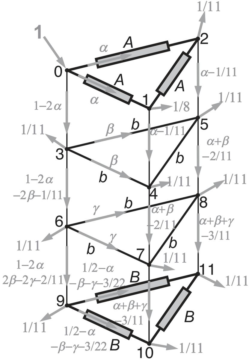
**Figure B1.** Equivalent diagram of an internal part of an  $m \times 3$  cylinder or globe network, displaying 12 internal nodes and two intermediate frame layers.
