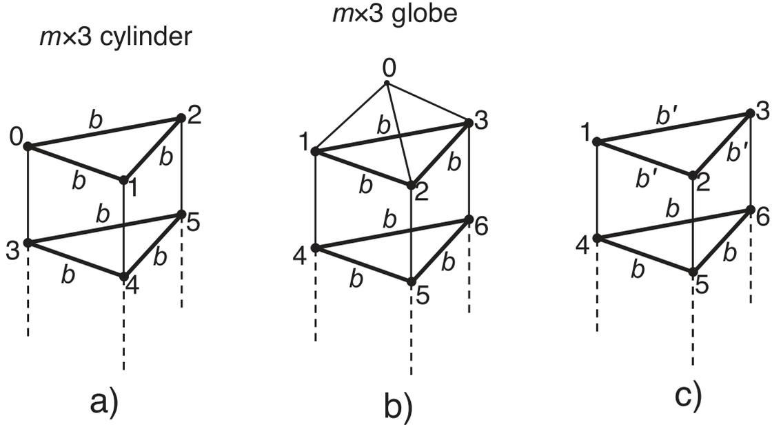
**Figure 2.** Upper parts of the  $m \times 3$  cylinder (a) or globe (b) networks. When the top node of the globe network is removed by applying the Y to  $\Delta$  transform, a cylinder network is obtained (c), but with a different resistor  $b'$  for the top frame instead of  $b$ .
