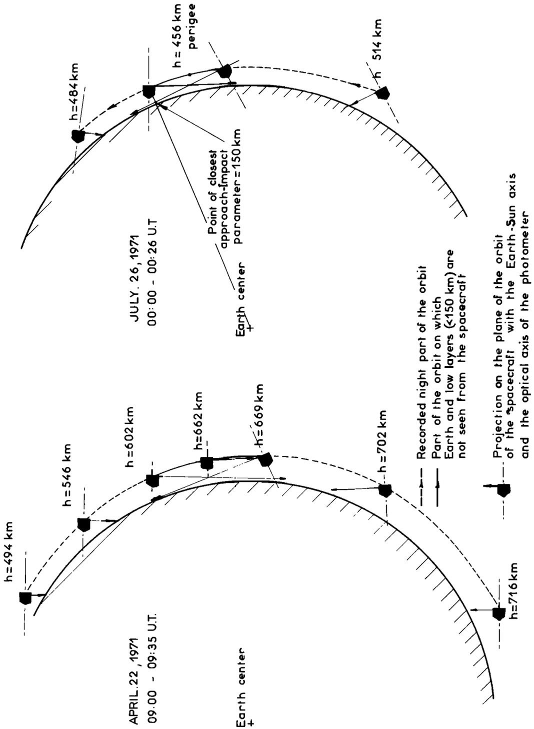
Fig. 2. Night part of D2A satellite orbits.
