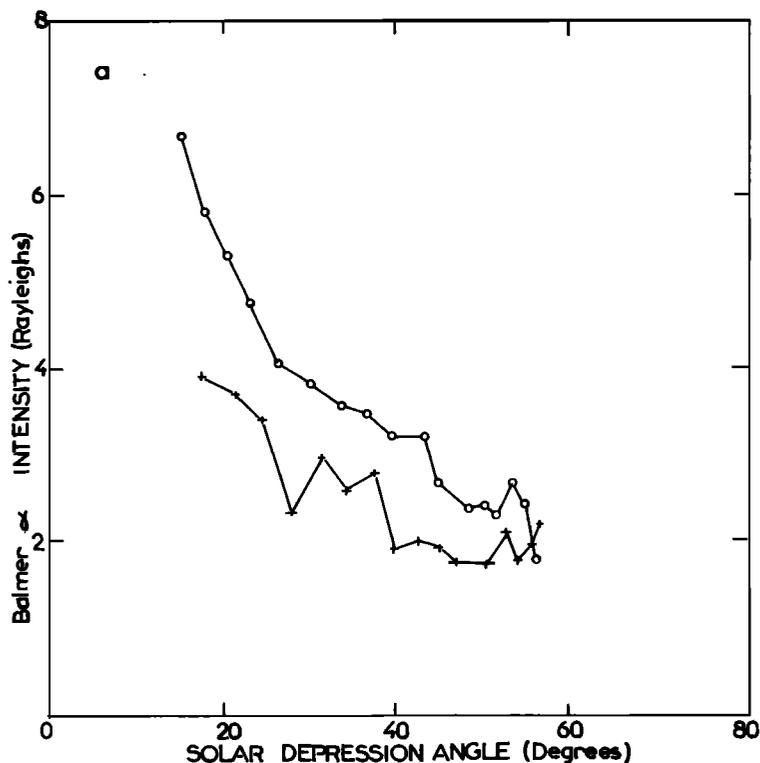
Fig. 7a. Average brightness of the geocoronal  $H\alpha$  emission perpendicular to the sun versus solar depression angle for the orbit on April 20, 1971. For the measurements taken into account the zenith distance was greater than  $45^\circ$ , and its average value for both orbits was equal to  $78^\circ$ . Data obtained before local midnight (crosses) and data obtained after local midnight (circles) are shown.
