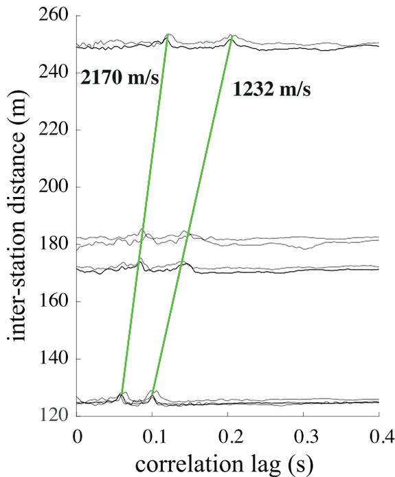
**Figure 3.** NCF from 8 h of seismic noise recorded between 0h00 and 8h00 on March 5, 2019 in the Van Mijen Fjord, at the stations of the array shown as blue squares in Figure 2c, versus the distance between the stations. The green lines indicate the arrival time of the  $QS_0$  and  $SH_0$  modes, which propagate at a velocity of 2,170 and 1,232 m/s, respectively.
