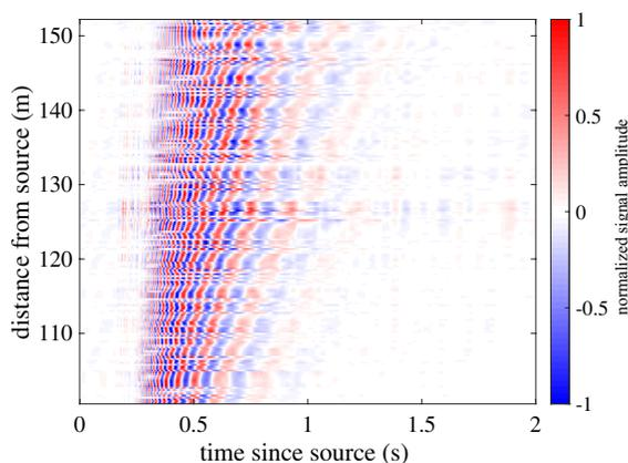
**Figure 4.** Normalized signals received at all stations of the main array versus the distance from an impulsive source located in the north linear array. Depending on propagation direction, the moveout of the waveforms is not increasing monotonically, revealing an apparent anisotropy of the wave propagation.
