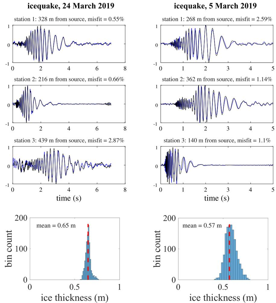
**Figure 6.** Top: waveforms of the icequakes recorded in the Van Mijen fjord (black) and the corresponding synthetic waveforms (blue), resulting from the inversion with 3 stations ( $S_1$ ,  $S_2$  and  $S_3$ ; see Figure 7). Bottom: PDF of the ice thickness, with the mean value shown as dashed line.
