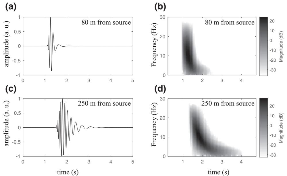
**Figure 1.** (a) Synthetic waveform of the QS mode received by a geophone located 80 m away from an impulsive source in a floating layer of ice with thickness 0.65 m. (b) Short-time Fourier transform of the waveform. (c) and (d) Same as (a) and (b) for a geophone located 250 m away from the source.
