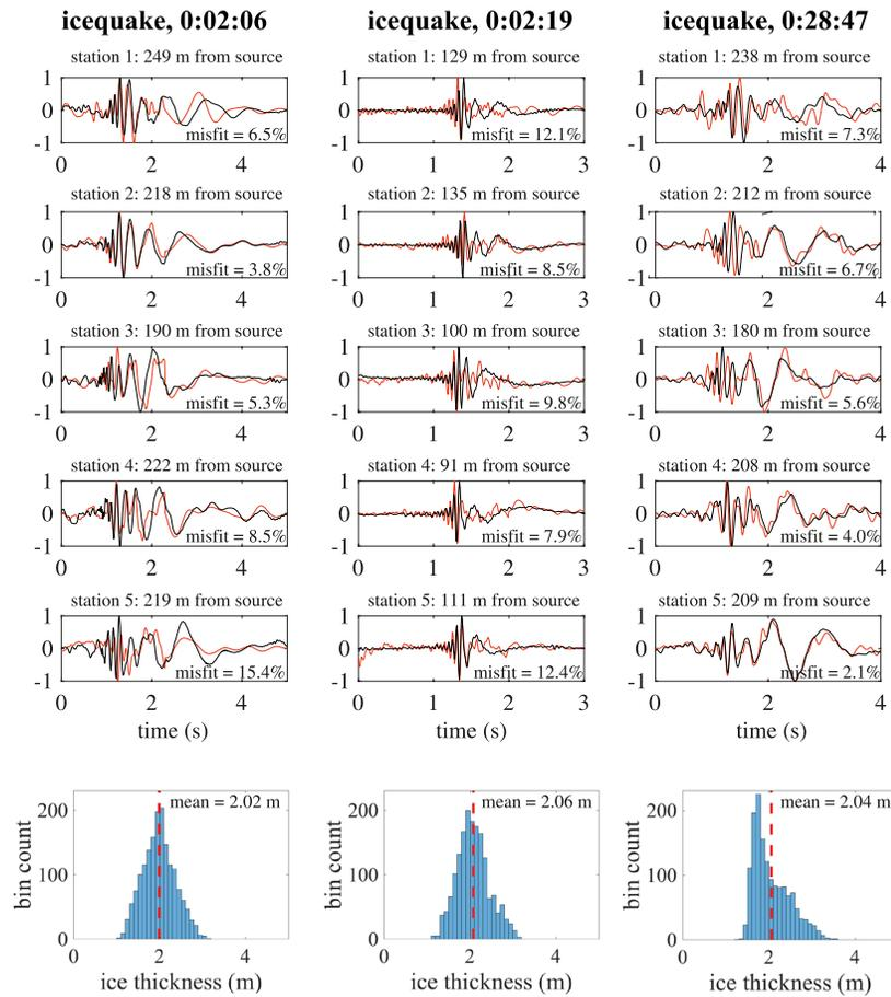
**Figure 10.** Top: Waveforms of the icequakes recorded on pack ice (black) and the corresponding synthetic waveforms (red), resulting from the inversion with 5 stations. Bottom: PDF of the ice thickness with the mean value shown as dashed line.
