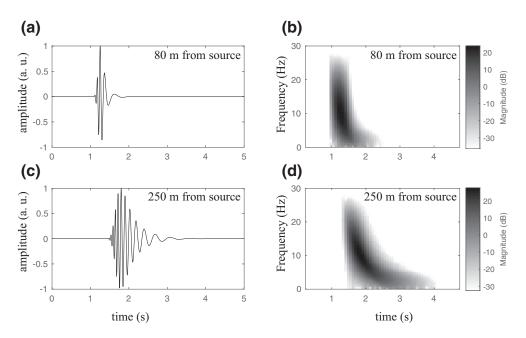
**Figure 1.** (a) Synthetic waveform of the *QS* mode received by a geophone located 80 m away from an impulsive source in a floating layer of ice with thickness 0.65 m. (b) Short-time Fourier transform of the waveform. (c) and (d) Same as (a) and (b) for a geophone located 250 m away from the source.
