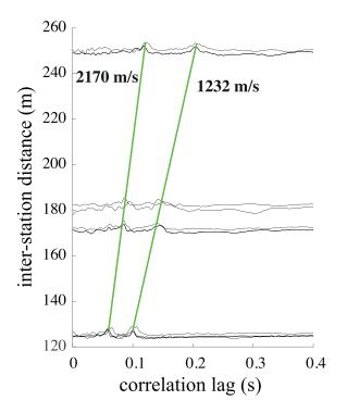
**Figure 3.** NCF from 8 h of seismic noise recorded between 0h00 and 8h00 on March 5, 2019 in the Van Mijen Fjord, at the stations of the array shown as blue squares in Figure 2c, versus the distance between the stations. The green lines indicate the arrival time of the  $QS_0$  and  $SH_0$  modes, which propagate at a velocity of 2,170 and 1,232 m/s, respectively.
