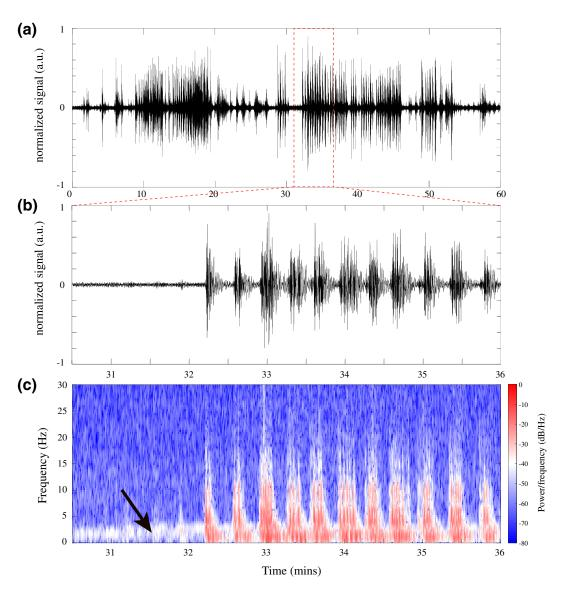
**Figure 9.** (a) One hour of seismic recording at one station of the HELSINKI antenna. (b) Zoom between 0:30:30 and 0:36:00 and (c) the corresponding short-time Fourier transform. The black arrow indicates a systematic seismic noise with energy between 0.5 and 3 Hz.
