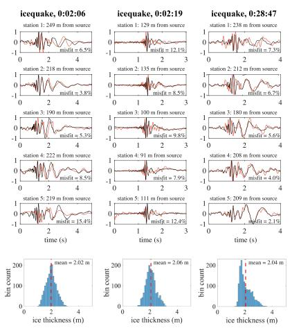
**Figure 10.** Top: Waveforms of the icequakes recorded on pack ice (black) and the corresponding synthetic waveforms (red), resulting from the inversion with 5 stations. Bottom: PDF of the ice thickness with the mean value shown as dashed line.
