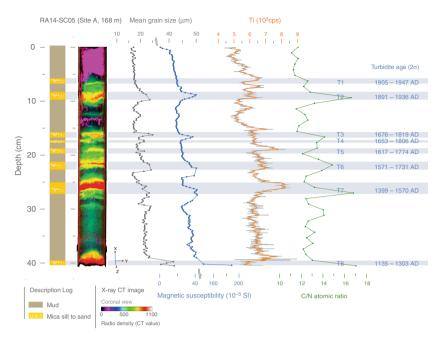
**Fig. 2** Identification of turbidites in sediment core RA14-SC05. From left to right are shown: a synthetic log, 3D coronal view of computed X-ray tomography images in pseudo-colour, mean grain size, magnetic susceptibility, Itrax XRF Ti profile (grey curve: raw data; orange curve: 5 pt-weighted average) and carbon to nitrogen (C/N) atomic ratio. These five parameters were used to identify turbidites T1 to T8. Their ages were extracted from the age-depth model (see Methods)
