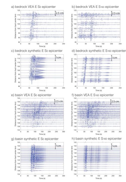
**Figure 7.** Displacement waveforms of the east component (approximately Rayleigh waves) for two scenario ruptures ([a, c, e, and g]  $S_0$  and [b, d, f, and h]  $S_{160}$ ; Figure 1 for selected bedrock sites, where the basement depth is shallower than 500 m). VEA = virtual earthquake approach.
