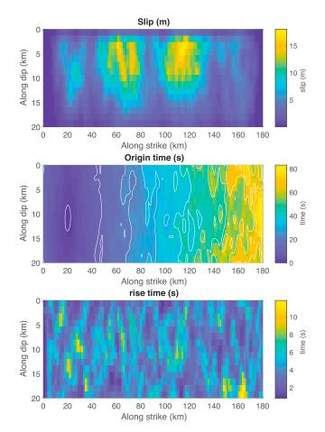
Figure 5. Representative example of a source model showing slip, rupture time, and rise time.
