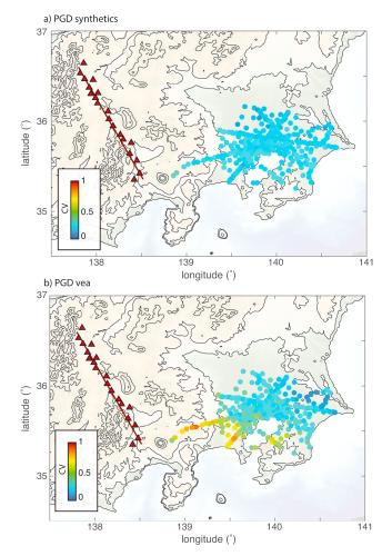
**Figure 11.** Coefficient of variation coefficient of variation of PGD for (a) synthetics and (b) VEA. Topography is shown in colorscale and extracted from topex.ucsd.edu (Smith & Sandwell, 1997). PGD = peak ground displacement; VEA = virtual earthquake approach.
