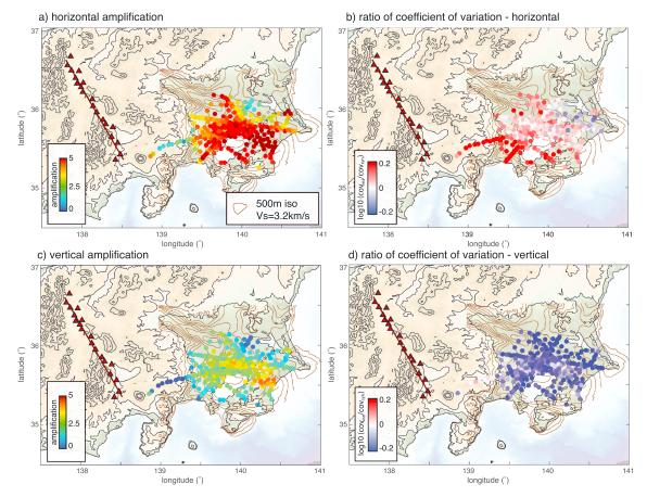
**Figure 13.** Comparison of the virtual earthquake approach displacements relative to 1-D synthetics for (a) peak ground displacement and (b) ratio of the coefficient of variation for horizontal components; (c) and (d) are same as in (a) and (b) but for vertical ground motions. Topography is shown in colorscale and extracted from topex.ucsd.edu (Smith & Sandwell, 1997) and basin contours are the iso  $V_s = 3.2$ -km/s contours (Koketsu et al., 2009).
