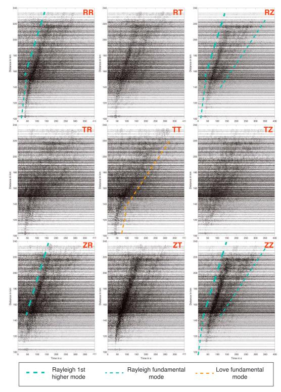
**Figure 2.** Averaged cross-correlation functions from virtual source SSWH to all Metropolitan Seismic Observation network stations and at all nine components of the Green tensor. The dash colored lines provide a crude indication of the move out of Love and Rayleigh wave fundamental modes and Rayleigh wave first higher modes.
