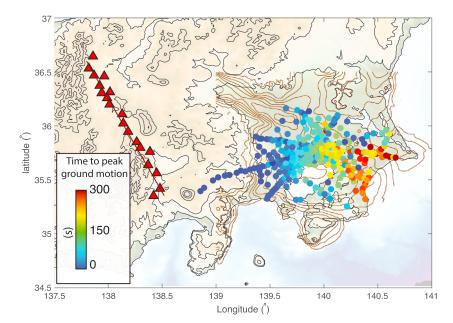
**Figure 16.** Time of the peak amplitude one scenario source  $S_{60}$ . Topography is shown in colorscale and extracted from topex.ucsd.edu (Smith & Sandwell, 1997), and basin contours are the iso  $V_S = 3.2$ -km/s contours (Koketsu et al., 2009).
