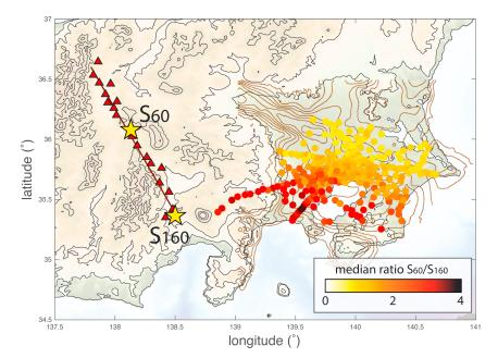
**Figure 18.** Median ratios of peak ground displacements from the scenario sources with the epicenter at the coupling point ( $S_{60}$ ) and at the southern edge of the fault model ( $S_{160}$ ). Topography is shown in colorscale and extracted from topex.ucsd.edu (Smith & Sandwell, 1997), and basin contours are the iso  $V_S = 3.2$ -km/s contours (Koketsu et al., 2009).
