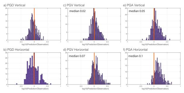
**Figure 4.** Histograms of the ratio of predicted and observed peak ground motion (horizontal and vertical) for the Nagano earthquake. Redline highlights an accurate prediction. (a) and (b) show the PGD fit, (c) and (d) show the PGV fits, and (e) and (f) show the PGA fits. PGA = peak ground acceleration; PGD = peak ground displacement; PGV = peak ground velocity.
