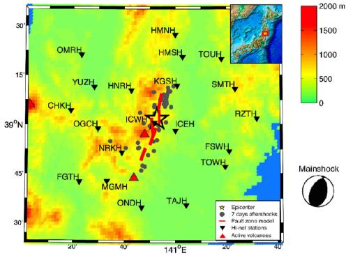
**Figure 1.** Map of the topography of the Iwate-Miyagi area. Black triangles: Hi-net stations; brown star: epicentre of the 2008 Iwate Miyagi earthquake; red lines: upper edges of the fault proposed by Takada *et al.* (2009); grey dots: aftershocks with magnitudes >3.5 within 7 d of the main earthquake and red triangles: active volcanoes. The beachball plot describes the source mechanism associated with the earthquake. Inset: position of the Iwate-Miyagi area within Japan.
