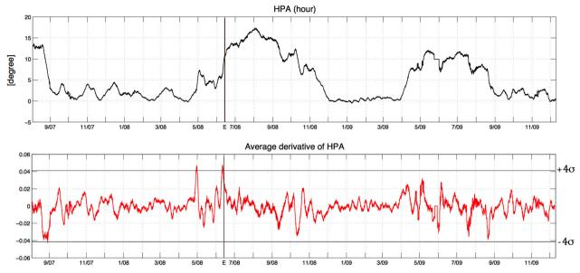
**Figure 3.** Top panel: average of the horizontal polarization anomaly from mid-2007 to the end of 2009. Bottom panel: the first derivative of the average horizontal polarization anomaly (red signal). The flat values at the end of 2009 May are due to a gap in the data. The variance  $\sigma$  of the average derivative of HPA has been computed for the whole period of study.
