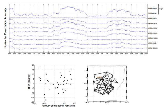
**Figure A4.** Top panel: example of temporal change in the horizontal polarization anomalies computed by the optimal rotation algorithm, for pairs of receivers for station HNRH. Bottom left panel: distribution of the HPA computed for all pairs of receivers as a function of the azimuth of the pairs. Bottom right panel: locations of the processed pairs of receivers.
