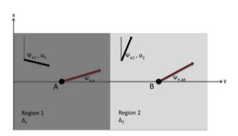
Figure A7. Map view of the two anisotropic regions around stations A and B.  $\Psi_{P,A}$  is the polarization anomaly of the wave arriving at station A and  $\Psi_{P,AB}$  is the final polarization anomaly of the wave propagating from A to В.
