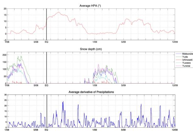
Figure 4. Top panel: average change in the horizontal polarization anomaly. Middle panel: seasonal changes in snow depth (from the Japan Meteorological Agency) in the area of study for 2008 and 2009. Bottom panel: average rainfall per week (from the Japan Meteorological Agency).
