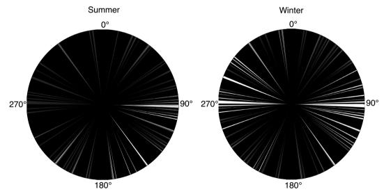
Figure A5. Polar plot of the azimuth of incidence of the noise in summer and winter relative to the area and time of the study, computed using the method described in Stehly *et al.* (2006). In the grey colour scale of the polar plots, white corresponds to the maximum amplitude of noise and black corresponds to the absence of noise.
