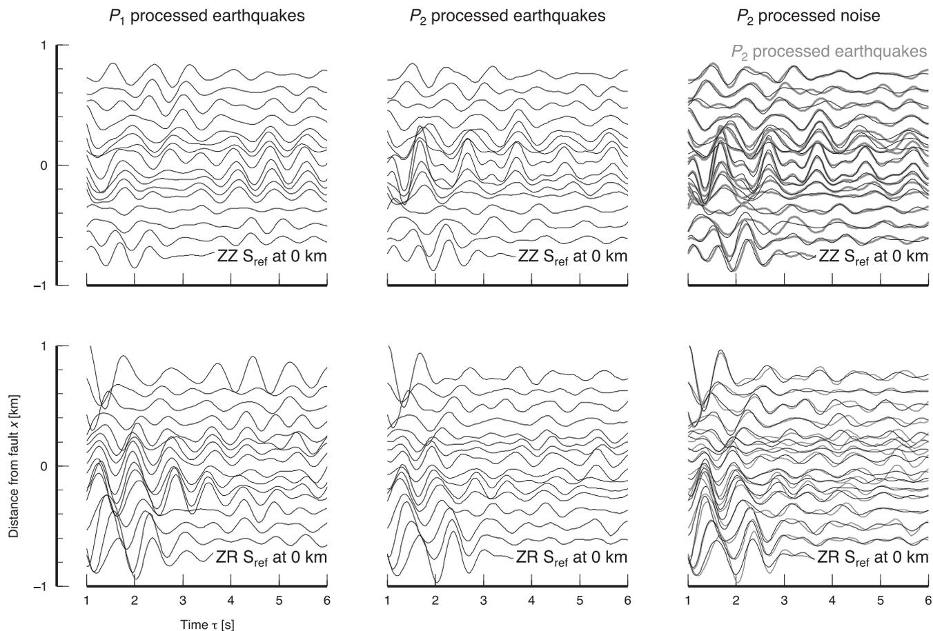
**Figure 7.** Lapse time or  $\tau$ -averaged correlation coda from  $P_1$  and  $P_2$  processed earthquake waveforms and noise. Panels in the top (bottom) row show ZZ (ZR) correlations. The images focus on the 2 km wide region around the mapped fault trace. In the right column, we plot seismograms from the middle column in grey to illustrate the waveform similarity.
