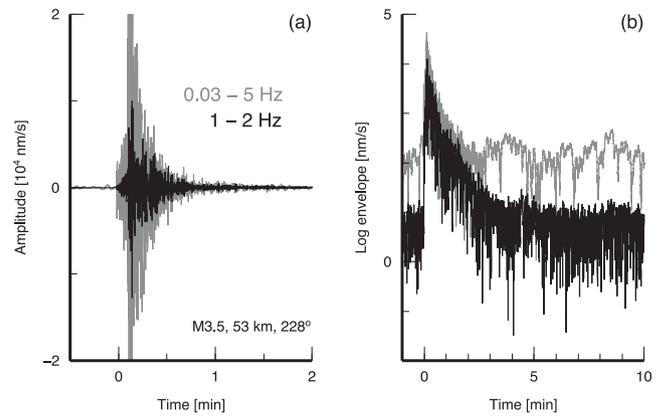
**Figure 3.** (a) Bandpass filtered seismograms of a regional M3.5 earthquake. (b) The envelopes of the filtered seismograms indicate an increased noise level at low frequencies. Coda energy is dissipated after 3–5 min in the 1–2 Hz target frequency range.
