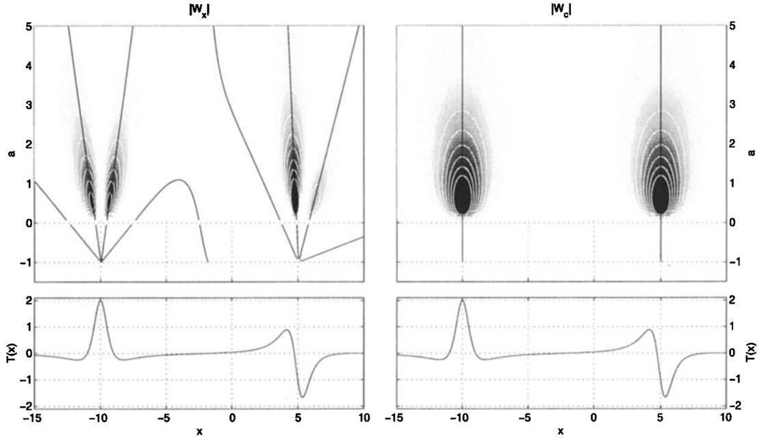
**Figure 5.** Local elementary magnetizations at depth  $z_0 = 1$  (and  $a = -z_0 = -1$ ) with apparent inclinations  $I' = 90^\circ$  at  $x = -10$  and  $I' = 29.16^\circ$  at  $x = +5$ : (bottom) Total magnetic field, and (left) modulus of real wavelet coefficients or (right) complex wavelet coefficients. Isovalues are shown in white with regular intervals. Modulus maxima lines are shown in black with their downward continuation to the source.
