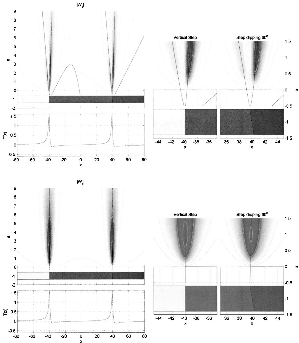
**Figure 7.** Vertical and dipping steps of magnetization (at mean depth  $z_0 = 1$ , with apparent inclination  $I' = 29.16^\circ$ ): (bottom left) Total magnetic field, and (top left) corresponding modulus of real or complex wavelet coefficients (zoomed at right). Isovalues are shown shaded with regular intervals. Modulus maxima lines are shown in black; their continuation to the source is shown in the lower half-space (analytically, above the top of the source).
