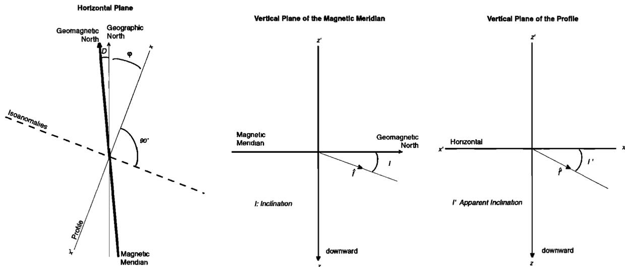
**Figure 4.** Apparent inclination  $I'$  versus inclination  $I$ : The unit vector  $\hat{f}$  (respective  $\hat{f}_n$ ) defining the direction of the magnetization  $M$  (respective of the magnetic field  $F$ ) gives the apparent inclination  $I'$  (respective  $I'_n$ ) when projected onto the vertical plane of the profile.
