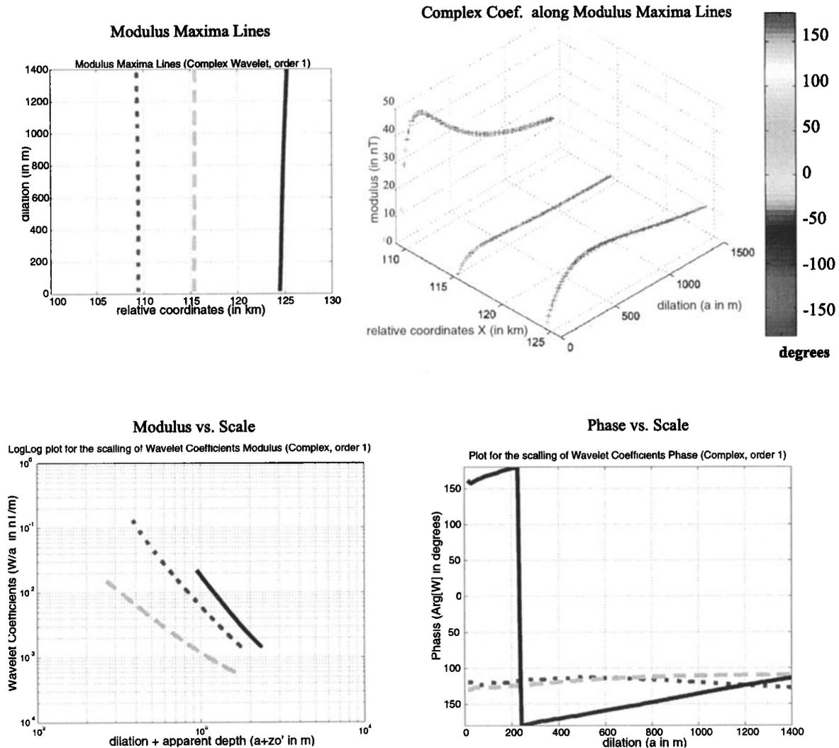
**Figure 14.** Characterization of the sources from the use of 1-D complex wavelets: (top) The modulus maxima lines and the phase along these lines obey (bottom) scaling relations characterizing the two dikes (dotted and dashed) and the fault (plain); (bottom left) homogeneity degree is given by the plot of  $\log(|W_a|/a)$  versus  $\log(a + z_0)$ , and (bottom right) inclination is given by the limit of  $\text{Arg}(W_a)$  for large  $a$ .
