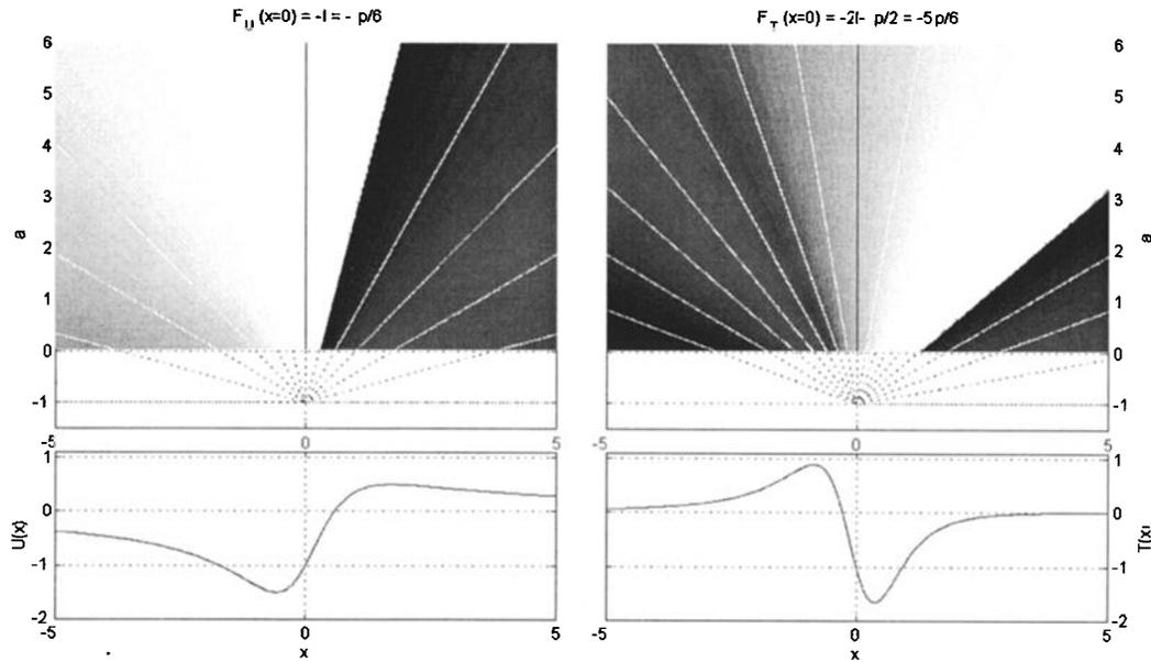
**Figure 3.** Magnetic potential  $U$  and total field  $T$  due to a dipole with inclination  $I = \pi/6$  at  $x_0 = 0$  and  $z_0 = 1$  analyzed with complex wavelet  $\psi_c^1$ : Phase isovalues (shown in white, every  $\pi/6$ ) converge to the source (dotted lines); the phase isovalue  $\Phi(x = 0)$  (for  $x = x_0 = 0$ ) gives the inclination  $I$ .
