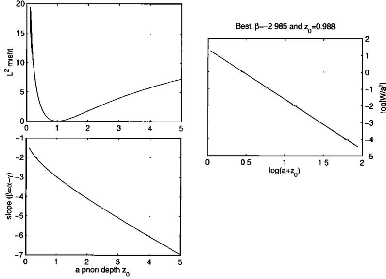
**Figure 6.** From the wavelet coefficients of Figure 5, (right) computation of the best slope  $\beta$  and depth  $z_0$  is accomplished by least squares linear regressions of  $\log(|W_a|/a^\gamma)$  versus  $\log(a + z_0)$ . (left) A set of a priori depths  $[0.1, 5]$  has been tested; this gives good estimates for both homogeneity degree  $\alpha = \beta + \gamma = -1.985$  and depth  $z_0 = 0.988$ .
