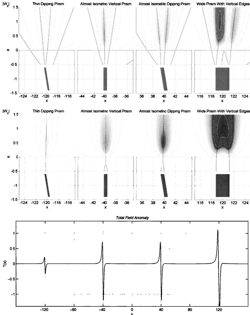
**Figure 9.** Vertical and dipping ( $\theta = -40^\circ$ ) prisms of magnetization (at depth  $z_0 = 1$ , with apparent inclination  $I' = 29.16^\circ$ ): (bottom) Total magnetic field and corresponding modulus of (top) real or (middle) complex wavelet coefficients. Isovalues are shown shaded with regular intervals. Modulus maxima lines are shown in black; their continuation down to the source is shown for small dilations in the lower half-space.
