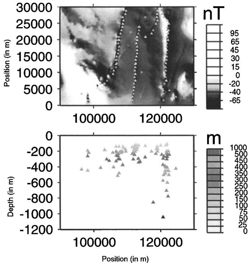
**Figure 13.** Imaging sources from the use of 1-D real wavelets: Each profile anomaly provides one source location. For the set of profiles in the area this maps horizontal positions and depths (top) as seen from above superimposed on the anomalies in grey scale and (bottom) its vertical cross section projection. For the central profile one gets the following depths  $z_0$  (from the SSW to the NNE): 370 m (SSW dike), 250 m (middle dike), and 930 m (the fault).
