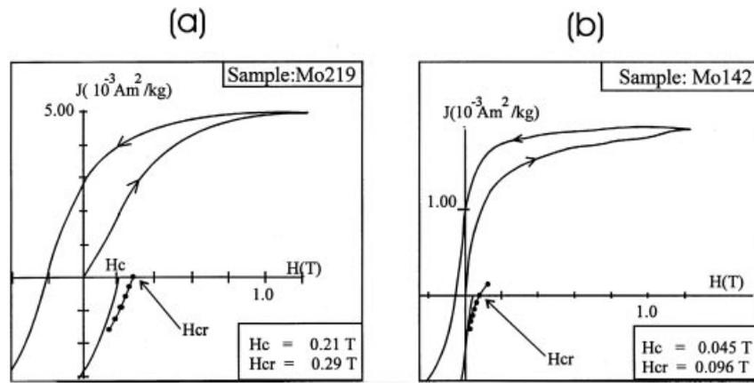
Figure 2. Hysteresis loop: (a) blue-violet limestone; (b) rubefied red clays ( $H_c$ : coercive force;  $H_{cr}$ : remanent coercive force).
