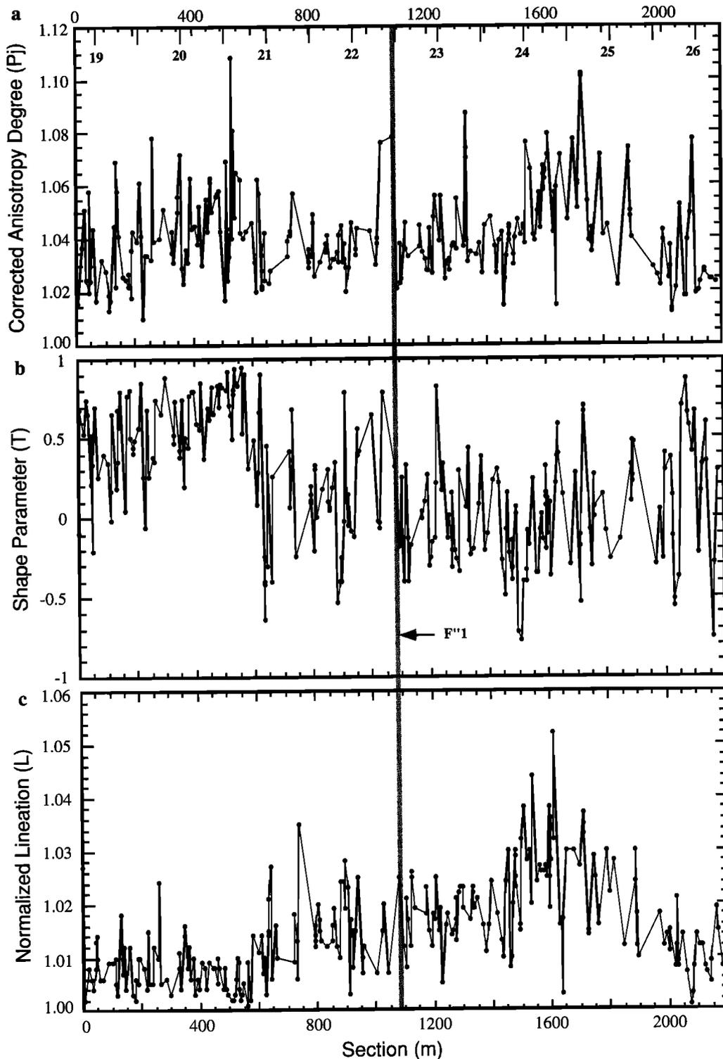
**Figure 10.** (a) Corrected anisotropy degree ( $P_j$ ) [Jelinek, 1981], (b) shape parameter ( $T$ ) ( $T < 0$  for prolate, pencil-like shapes;  $T > 0$  for oblate, pancake-like shapes), and (c) normalized lineation ( $L$ ) [e.g., Hrouda, 1982] plotted against depth (0 is top; 2179 m is bottom). Scale in Ma from correlation II of Figure 5 is provided in Figure 10a.
