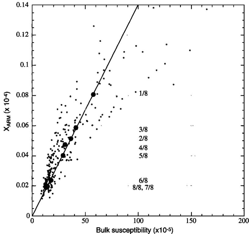
**Figure 9.** Normalized anhysteretic remanent magnetization intensity plotted against  $k$  (open circles). Solid circles are mean values of each eighth of the section (1/8 is top; 8/8 is bottom). Note that mean values lie on the same slope.
