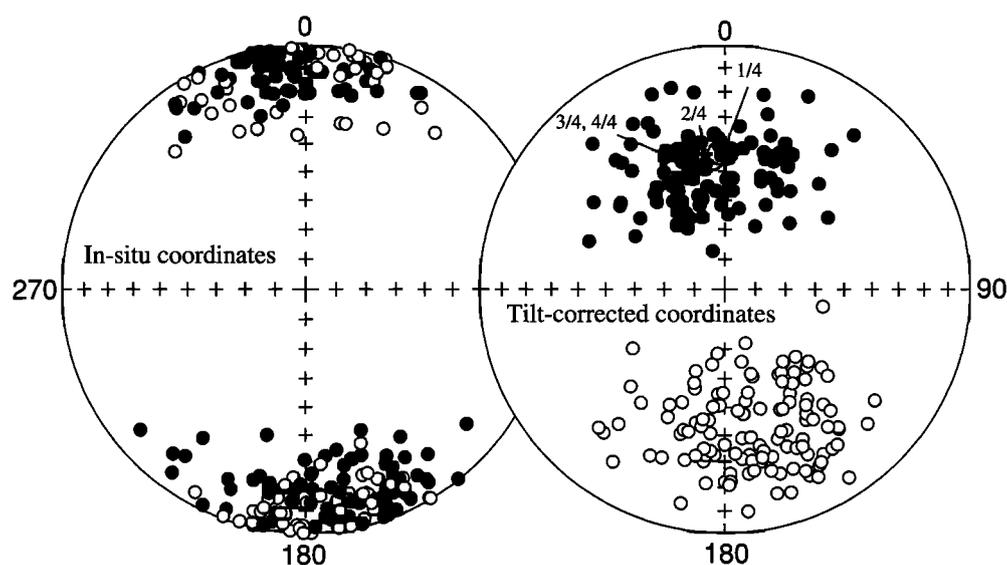
**Figure 4.** Stereonet plot of 222 magnetization directions used to constrain the magnetostratigraphy shown in Figure 5. Open (solid) circles are projected on the upper (lower) hemisphere. Stars and 95% confidence ellipses are mean values of each quarter of the section (1/4 is top; 4/4 is bottom) (data from Table 1).
