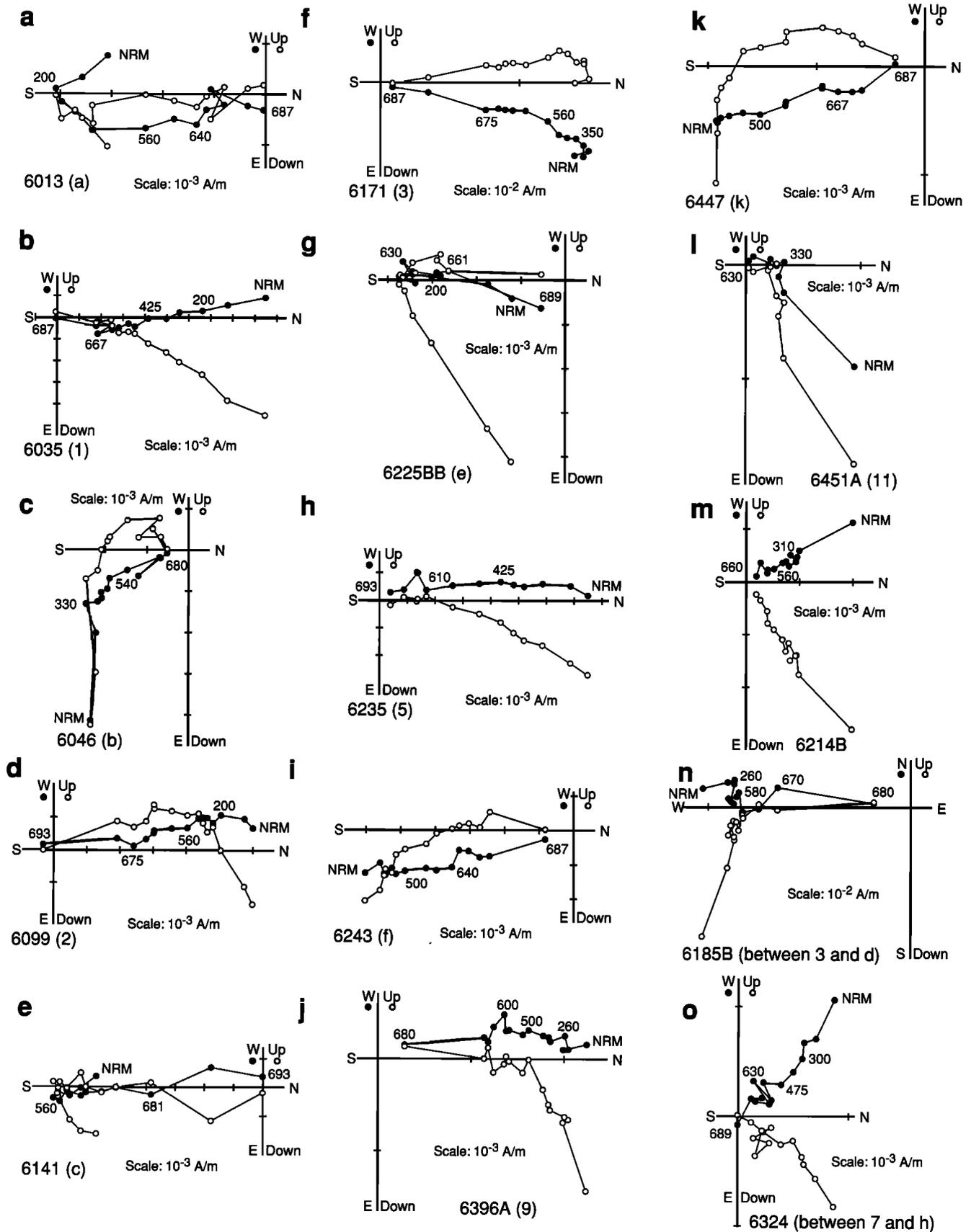
**Figure 3.** *Zijdeveld* [1967] plots from thermal demagnetization experiments (all in in situ coordinates). Numbers next to demagnetization steps are temperatures in degrees Celsius; natural remanent magnetization (NRM) is the room temperature step. Numbers at bottom left of plots are sample numbers (6001 is top of section, 6545 is bottom); numbers and letters in parentheses correspond to polarity sequences shown in Figure 5.
