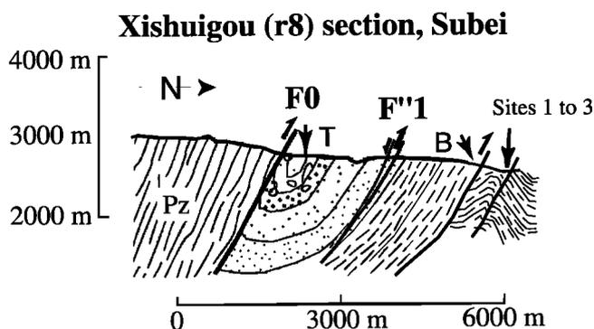
**Figure 2.** Simplified cross section of the Xishuigou (r8) section at Subei [after Van der Woerd et al., this issue]. Arrows show top (T) and bottom (B) of magnetostratigraphic section from this study. Transition from fine- to coarse-grained sediments is schematic. Pz represents Paleozoic metamorphic rocks.
