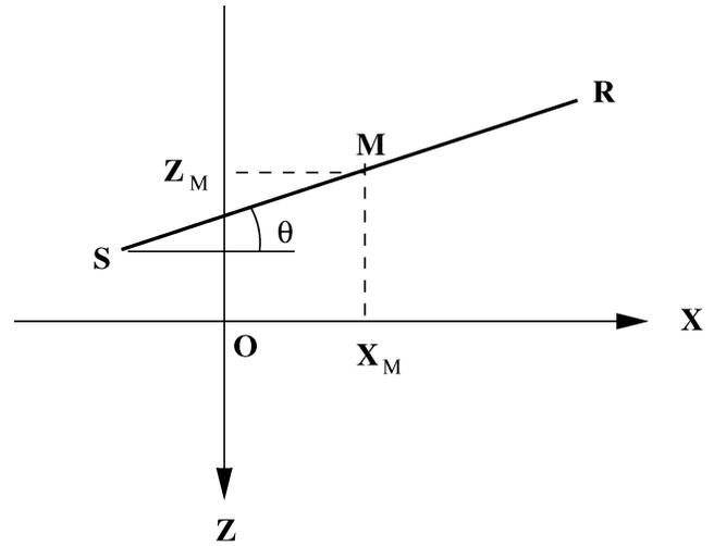
**Figure 1.** Geometrical parameters for 2-D tomography. The source–receiver pair  $(S, R)$  is uniquely defined by four parameters:  $X$  and  $Z$  positions of the mid-point  $M$ , the orientation  $\theta$  with respect to the  $X$ -axis, and the source–receiver distance  $d(R, S)$ .
