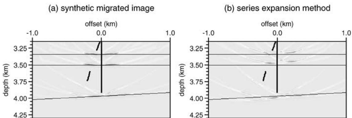
**Figure 7.** Diffraction pre-stack migration without aperture limitation. (a) Synthetic migrated image. (b) Migrated image processing times grid computed with the series expansion. The series expansion migration is five times faster than ray-tracing migration.
