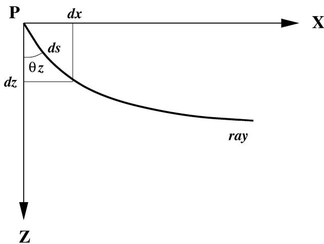
**Figure 2.** The incidence angle of the ray at  $P$ ,  $\theta_z$ , defined as the angle between the ray and the vertical axis, is computed from the ray parameter  $\mathbf{p}$  and the slowness  $s(P)$ .
