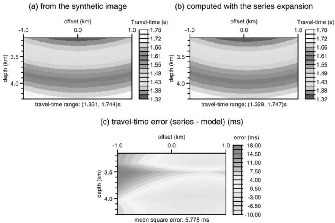
**Figure 6.** Traveltimes between the source at 0.0 km and 101 by 231 subsurface points located between  $-1.0$  and  $1.0$  km offset, and  $3.1$  and  $4.3$  km depth. Times calculated by (a) ray tracing through the true model, (b) times computed with the series expansion and (c) the error in traveltimes computation.
