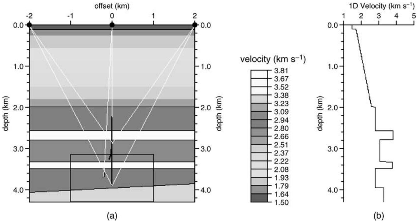
**Figure 3.** Synthetic velocity model and recording geometry. The velocity model is decomposed into eight layers. The velocity is constant in each layer except in the second layer in which the velocity increases linearly with depth. The velocity log at 0.0 km is plotted on the right of the figure. The acquisition geometry consists of three sources on the surface (black dots) and receivers in a borehole located at 0.0 km. The area between the white lines shows the ray coverage.
