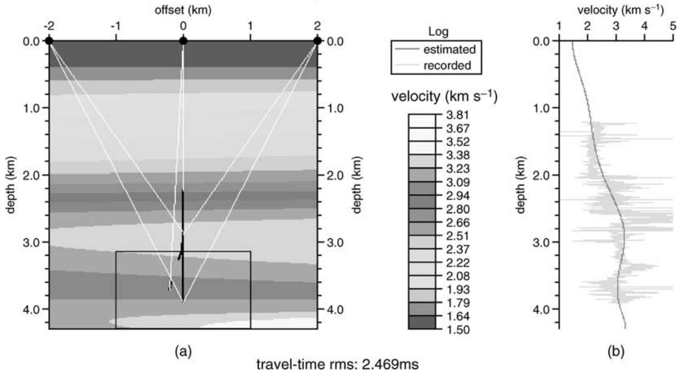
Figure 9. Velocity–depth model resulting from the series expansion tomography. The transmitted times are inverted with *a priori* information on the velocity given by the well log. The estimated log (dashed line) matches the sonic log (solid line).
