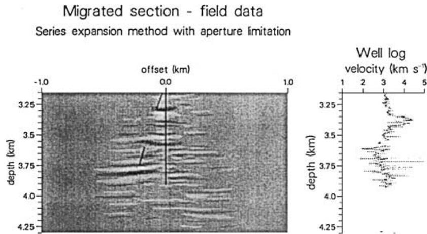
**Figure 12.** Diffraction pre-stack migration with an aperture limitation of  $15^\circ$ . The correlation between the migrated section and the recorded log plotted on the right, reveals that events are shifted up by 2 per cent compared with their expected locations given by the well log.
