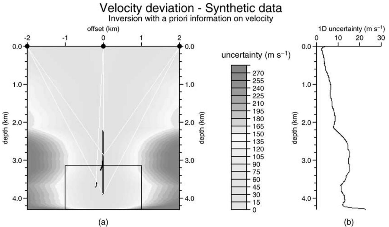
**Figure 5.** Uncertainty on the velocity reconstruction. The velocity at the vertical of the borehole is well resolved by the zero offset data. Uncertainty is limited to  $150 \text{ m s}^{-1}$  within the region covered by the rays and increases rapidly where data are not available.
