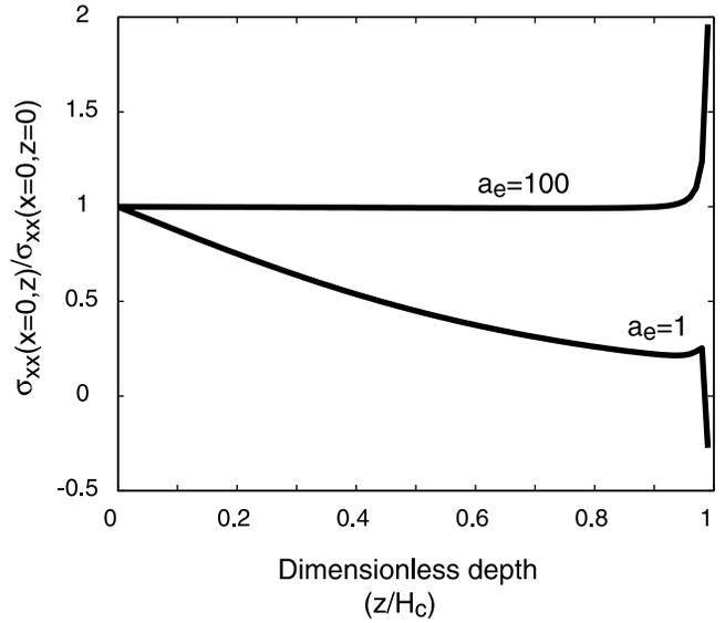
**Figure 5.** Horizontal normal stress  $\sigma_{xx}$  on the axis as a function of depth due solely to the edifice load at Earth's surface for a small reservoir ( $a_c = R_c/H_c = 0.01$ ). Calculations are made for a slab. Two curves are shown for two values of the dimensionless edifice radius  $a_e = R_e/H_c$ . For large  $a_e$ , the edifice generates compression over a large depth range and normal stress  $\sigma_{xx}$  remains constant at shallow depth above the reservoir.
