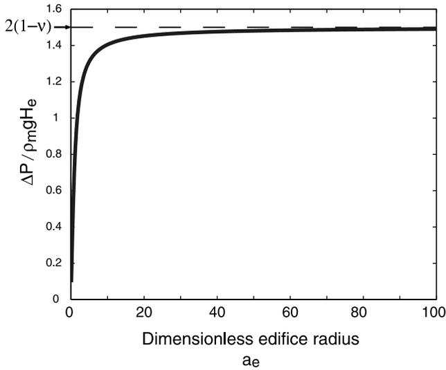
**Figure 4.** Magmatic overpressure required to achieve zero displacement of the reservoir walls beneath an edifice, as a function of dimensionless edifice radius  $a_e$  (equal to  $R_e/H_c$ ). Calculations are made for a slab. The dimensionless reservoir radius ( $a_c = R_c/H_c$ ) is set at 0.01. The overpressure tends to the constant value  $2(1 - \nu)\rho_m g H_e$  corresponding to the analytical solution for a cavity in an infinite medium.
