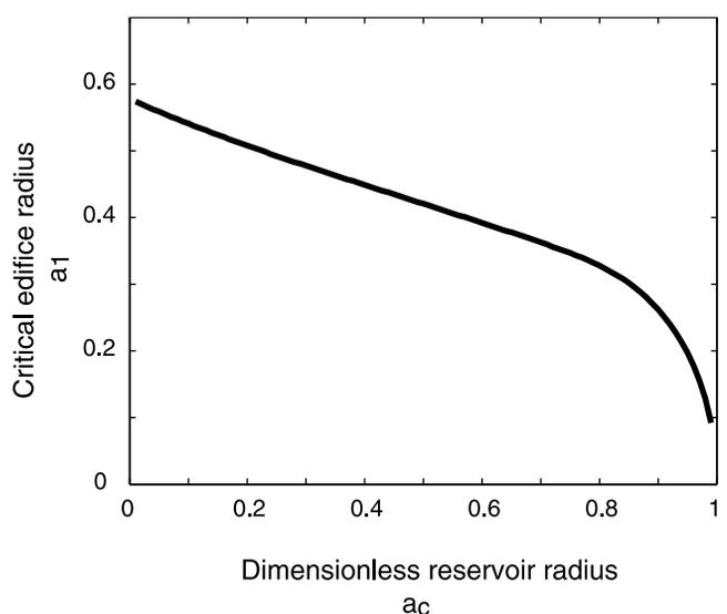
**Figure 10.** Critical value  $a_1$  of the dimensionless edifice radius  $a_e$  for which the magnitude of the tensile hoop stress reaches a maximum (see Figure 9), as a function of dimensionless reservoir size  $a_c$ .
