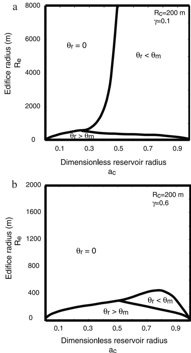
**Figure 12.** Values of the rupture angle  $\theta_r$  where the reservoir wall fails in tension for a small reservoir ( $R_c = 200$  m), as a function of edifice radius and dimensionless reservoir size  $a_c$ . (a) Shield volcano with gentle slopes ( $\gamma = 0.1$ ). (b) Stratovolcano with steep slopes ( $\gamma = 0.6$ ).
