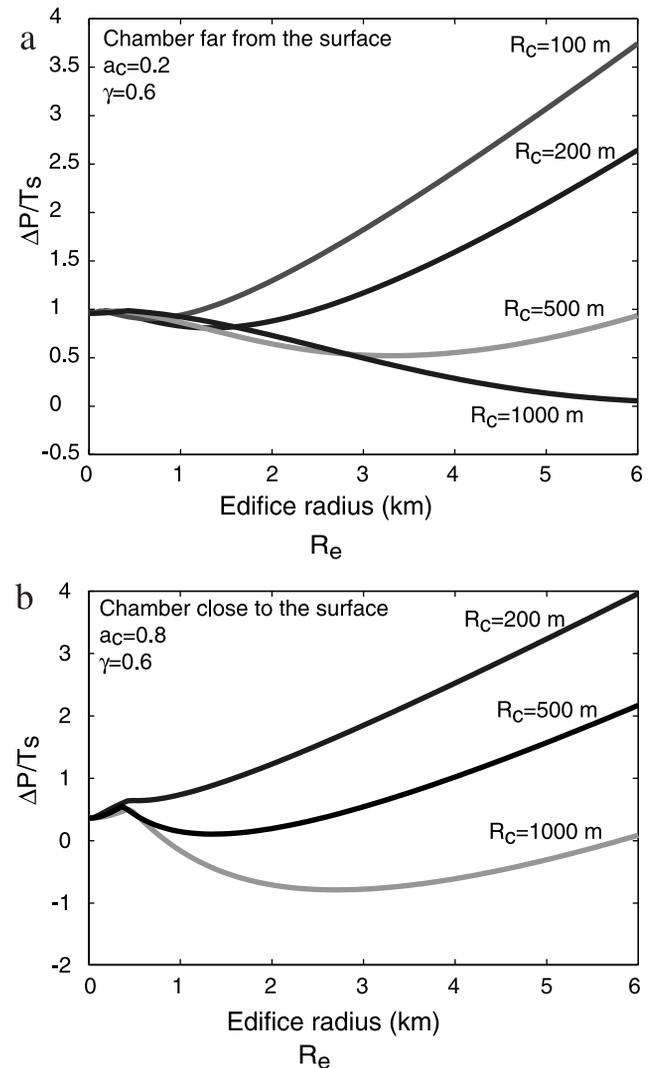
**Figure 14.** Critical magmatic overpressure for eruption as a function of edifice radius for a stratovolcano ( $\gamma = 0.6$ ). (a) Results for a deep reservoir ( $a_c = 0.2$ ). (b) Results for a shallow reservoir ( $a_c = 0.8$ ).
