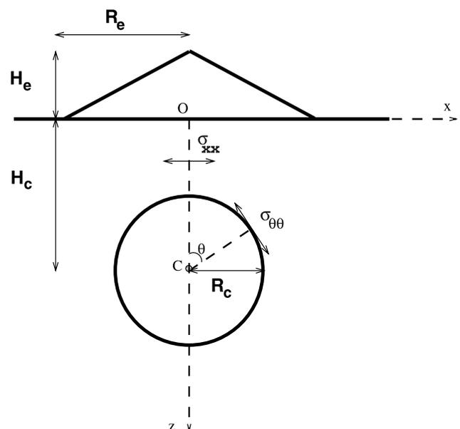
**Figure 2.** Geometrical setup for the problem. A cylindrical reservoir of radius  $R_c$  is located at depth  $H_c$  beneath a volcanic edifice. Angle  $\theta$  is measured with respect to the vertical axis of symmetry.  $\sigma_{\theta\theta}$  stands for the hoop stress on the reservoir walls. The volcanic edifice may be either a stratovolcano with steep slopes ( $\gamma = H_e/R_e = 0.6$ ) or a shield volcano with gentle slopes ( $\gamma = H_e/R_e = 0.1$ ).
