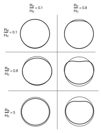
**Figure 11.** Displacement of the reservoir walls for the same cases illustrated in Figure 8. Displacement values have been multiplied by a factor of 5. Note the different results for small and large reservoir radii.
