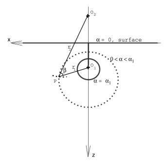
**Figure A1.** Bipolar coordinates for a half-space with a cylindrical cavity.
