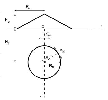
**Figure 2.** Geometrical setup for the problem. A cylindrical reservoir of radius  $R_c$  is located at depth  $H_c$  beneath a volcanic edifice. Angle  $\theta$  is measured with respect to the vertical axis of symmetry.  $\sigma_{\theta\theta}$  stands for the hoop stress on the reservoir walls. The volcanic edifice may be either a stratovolcano with steep slopes ( $\gamma = H_e/R_e = 0.6$ ) or a shield volcano with gentle slopes ( $\gamma = H_e/R_e = 0.1$ ).
