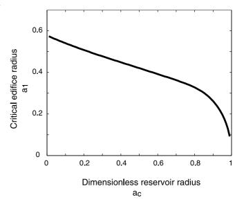
**Figure 10.** Critical value  $a_1$  of the dimensionless edifice radius  $a_e$  for which the magnitude of the tensile hoop stress reaches a maximum (see Figure 9), as a function of dimensionless reservoir size  $a_c$ .
