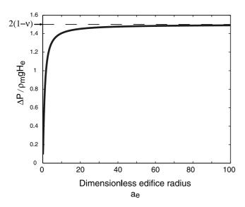
**Figure 4.** Magmatic overpressure required to achieve zero displacement of the reservoir walls beneath an edifice, as a function of dimensionless edifice radius  $a_e$  (equal to  $R_e/H_c$ ). Calculations are made for a slab. The dimensionless reservoir radius ( $a_c = R_c/H_c$ ) is set at 0.01. The overpressure tends to the constant value  $2(1 - \nu)\rho_m g H_e$  corresponding to the analytical solution for a cavity in an infinite medium.
