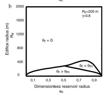
**Figure 12.** Values of the rupture angle  $\theta_r$  where the reservoir wall fails in tension for a small reservoir ( $R_c = 200$  m), as a function of edifice radius and dimensionless reservoir size  $a_c$ . (a) Shield volcano with gentle slopes ( $\gamma = 0.1$ ). (b) Stratovolcano with steep slopes ( $\gamma = 0.6$ ).
