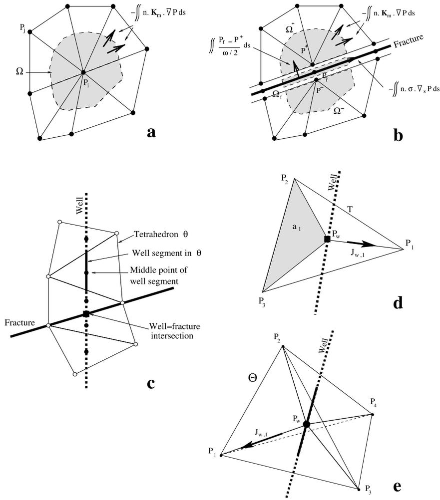
**Figure 2.** Control volumes around a point in the matrix (a) and on a fracture (b). Two-dimensional illustration of the introduction of the well in the mesh (c). Well intersection with a fracture surface element (d), and with a matrix volume element (e).
