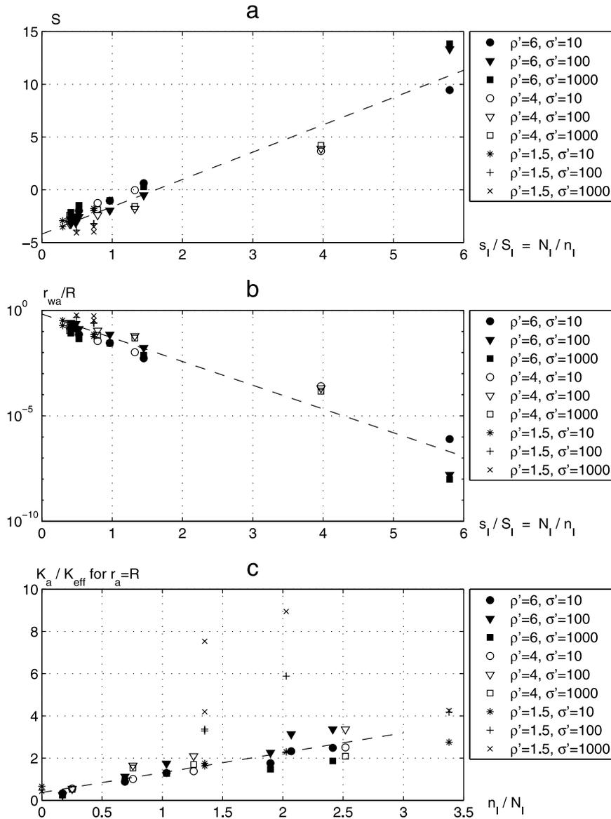
**Figure 9.** Coefficient  $S$  (a) and apparent well radius  $r'_{w,a}$  (b) as functions of the spacing  $s_1/S_1$ ; permeability ratio  $K_a/K_{eff}$  for  $r_a = R$  as a function of the number of intersections  $n_1/N_1$  (c). Data are for a well with a radius  $r_w = R/100$  in a randomly fractured medium, with various densities  $\rho'$  and fracture conductivities  $\sigma'$ . The broken lines correspond to the fit (47) in Figures 9a and 9b and to the fit (50) in Figure 9c.
