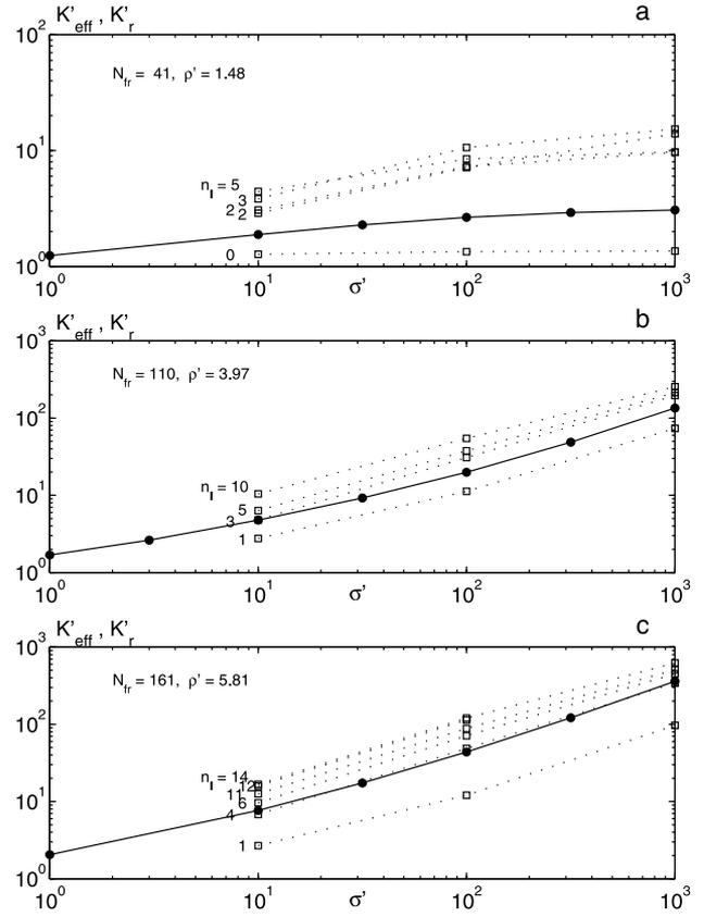
**Figure 8.** Effective permeability  $K_{eff}'$  (solid circles) and apparent permeability  $K_r'$  (open squares) for fractured media with  $\rho' = 1.48$  (a),  $3.97$  (b) and  $5.81$  (c), as functions of the fracture conductivity  $\sigma'$ . Data are for a unit cell size  $L = 6R$  and various numbers  $n_I$  of intersections of the well with the fracture network.
