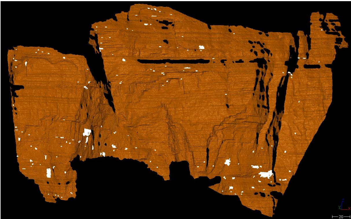
3 Figure 5. Upper: Mesh for the left scene 2012 and rockfall detected (white spots). Lower: Mesh 4 for the right scene 2012 and rockfall detected (white spots).
