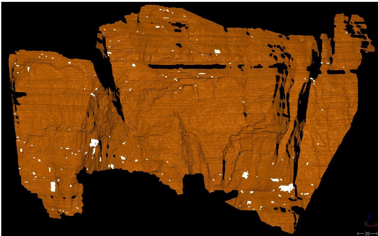
Figure 5. Upper: Mesh for the left scene 2012 and rockfall detected (white spots). Lower: Mesh for the right scene 2012 and rockfall detected (white spots).
