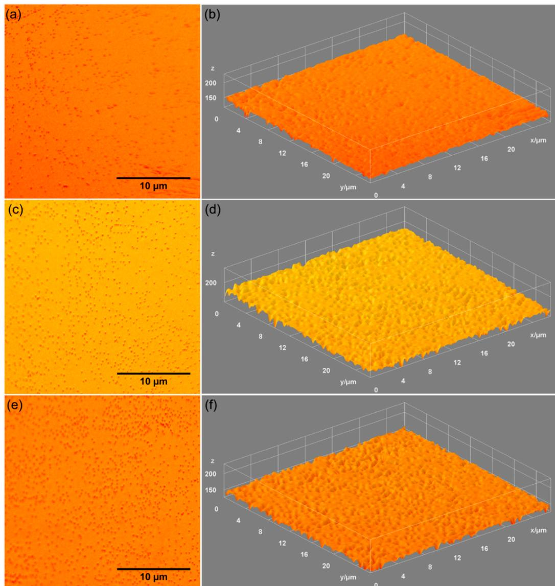
**Figure 4.** 2D Metallographic images (taken using 10× magnification) of HAp (a), 0.05 AgHAp (c), and 0.1 AgHAp (e) coatings, and 3D representation of the metallographic images of HAp (b), 0.05 AgHAp (d), and 0.1 AgHAp (f) coatings.
