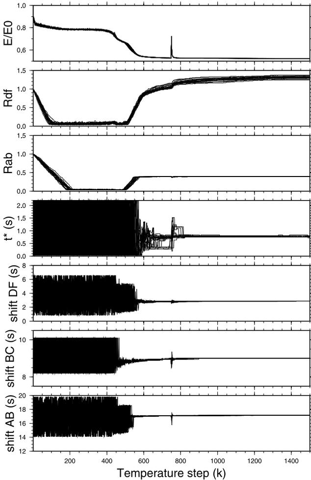
**Figure 5.** Energy,  $R_{DF}$ ,  $R_{AB}$  and parameters of a randomly selected seismogram for the 20 SA inversions, as a function of the temperature step ( $k$ ) describing the cooling schedule. From top to bottom: energy normalized to its starting value  $[E(k)/E(0)]$ ,  $R_{DF}$ ,  $R_{AB}$ , parameter  $t_1^*$  in seconds, and parameters  $\tau_1^{DF}$ ,  $\tau_1^{BC}$ , and  $\tau_1^{AB}$  in seconds.
