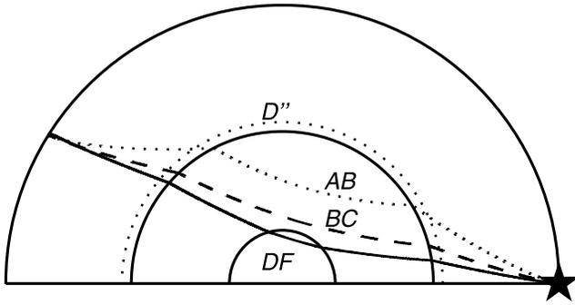
**Figure 1.** Ray paths of the three PKP branches in the Earth: PKP(DF) (solid line), PKP(BC) (dashed line) and PKP(AB) (dotted line). The event (black star) and the D'' layer at the base of the mantle are also indicated.
