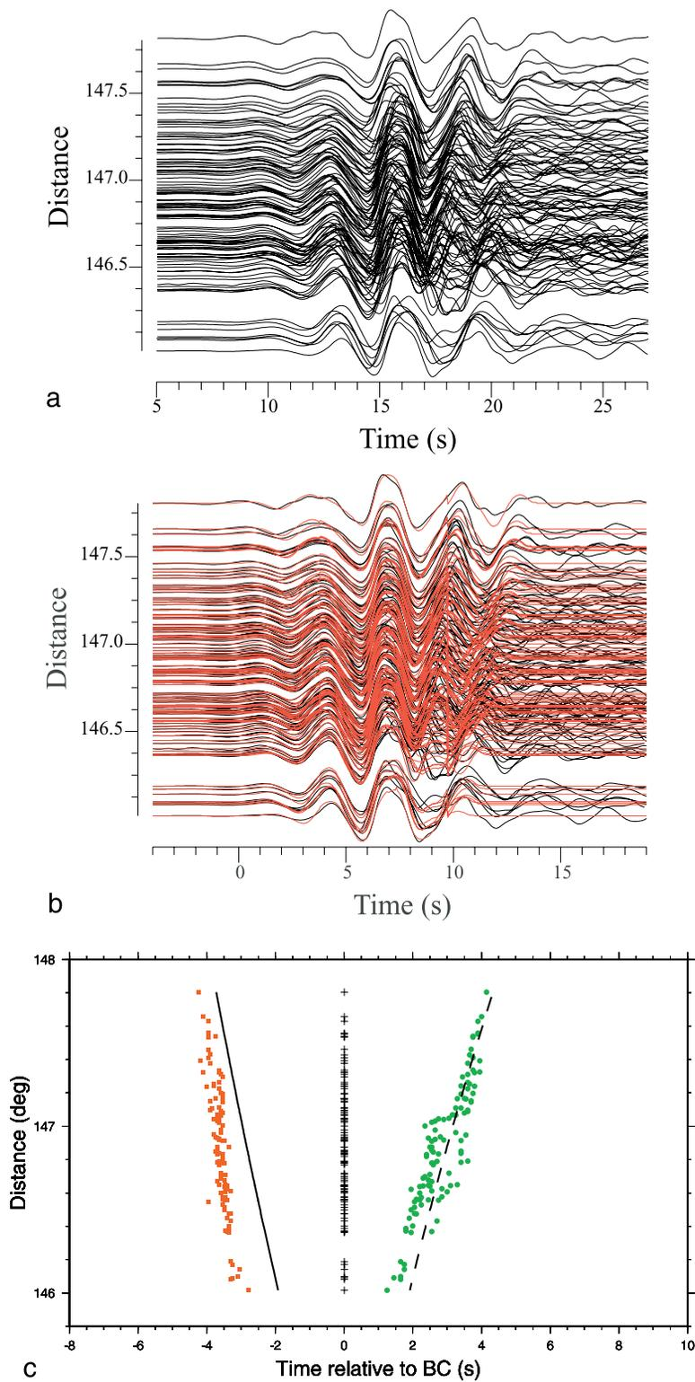
**Figure 7.** Example 2. (a) Raw data before inversion, aligned on the theoretical arrival time of  $PKP(BC)$ , and plotted as a function of their epicentral distance (in degrees). (b) Data (black lines) and best model synthetic seismograms (red lines) aligned on the  $PKP(BC)$  phase. (c) Best model arrival times of the three  $PKP$  phases relative to  $PKP(BC)$ . Dashed lines indicate theoretical arrival times predicted by the ak135 reference Earth's model.
