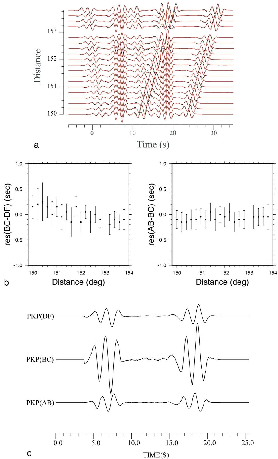
**Figure 8.** Nonlinear analysis of synthetic *PKP* data computed with the WKBJ software for an earthquake at 35 km depth. (a) WKBJ synthetic seismograms (black lines) and best model synthetic seismograms (red lines) aligned on the *PKP(BC)* phase. (b) BC-DF and AB-DF best model residuals as a function of epicentral distance. (c) From top to bottom, output *PKP(DF)*, *PKP(BC)*, and *PKP(AB)* waveforms including both the direct *PKP* phase and the corresponding  $p$ *PKP* depth phase.
