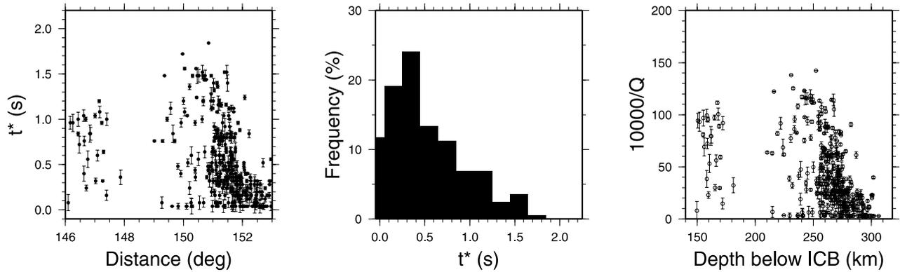
**Figure 13.** (left) BC-DF differential attenuation parameters  $t^*$  (s) as a function of epicentral distance ( $^{\circ}$ ). (middle) Histogram of BC-DF differential attenuation parameters  $t^*$ . (right) Inner core attenuation parameter  $q = 10,000/Q$  is shown as a function of depth of the *PKP*(DF) turning point in the inner core (km). Over the whole Eifel core phase data set, only  $t^*$  parameters presenting statistical errors lower than 0.1 s are plotted.
