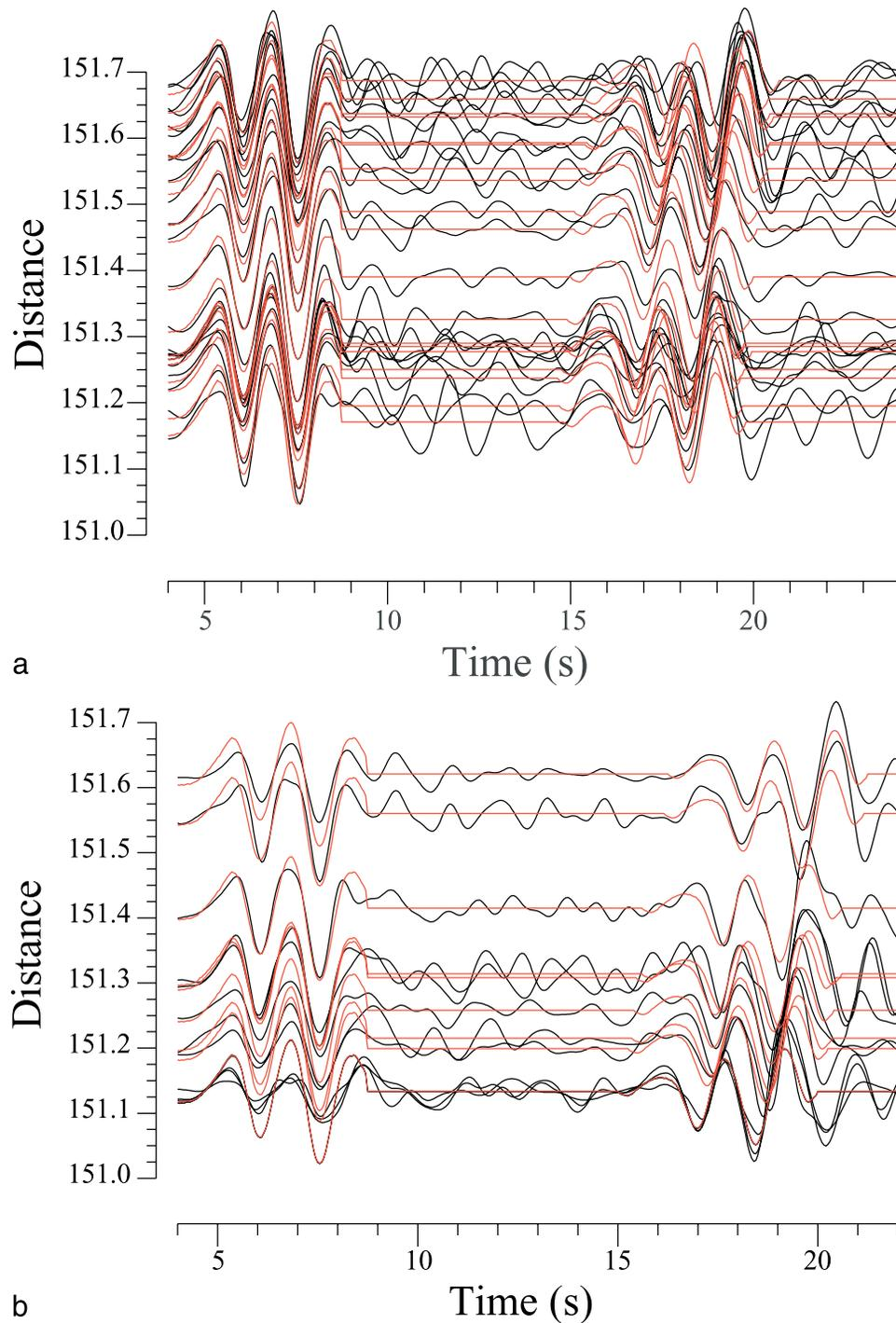
**Figure 11.** Closeup on the records of event 8 presenting (a) nominal  $PKP(AB)$  arrivals on top and (b) late arrivals on the bottom. Data (black lines) and synthetics (red lines) are aligned on the  $PKP(BC)$  phase seen on the left of the record sections. The  $PKP(AB)$  phase is properly fitted on both plots demonstrating that the larger AB-BC residuals are not due to cycle skipping problems. A similar pattern is observed for the AB-BC anomalous residuals of events 2 and 3.
