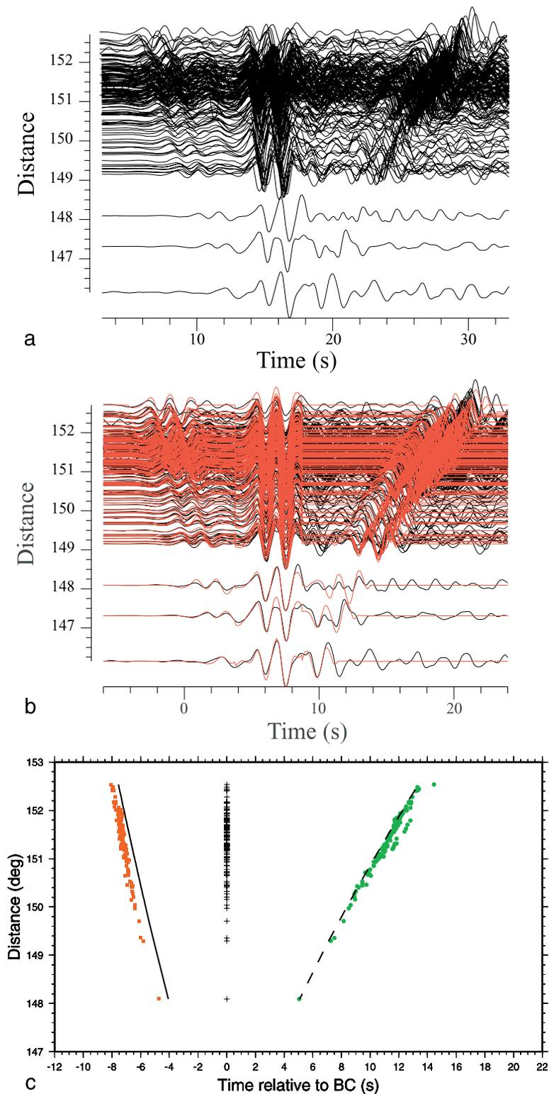
**Figure 3.** Example 1. (a) Raw data before inversion, aligned on the theoretical arrival time of  $PKP(BC)$  and plotted as a function of their epicentral distance (in degrees). (b) Data (black lines) and best model synthetic seismograms (red lines) aligned on the  $PKP(BC)$  phase. (c) Best model arrival times of the three  $PKP$  phases relative to  $PKP(BC)$ . Dashed lines indicate theoretical arrival times predicted by the ak135 reference Earth's model.
