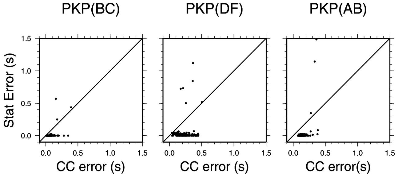
**Figure 4.** Statistical estimate of the time shifts RMS errors (in seconds) plotted as a function of the error computed for the best model using the cross correlation method described by *Chevrot* [2002]. From left to right, errors of the parameters  $\tau_i^{BC}$ ,  $\tau_i^{DF}$ , and  $\tau_i^{AB}$ . The line indicates the one to one correspondence.
