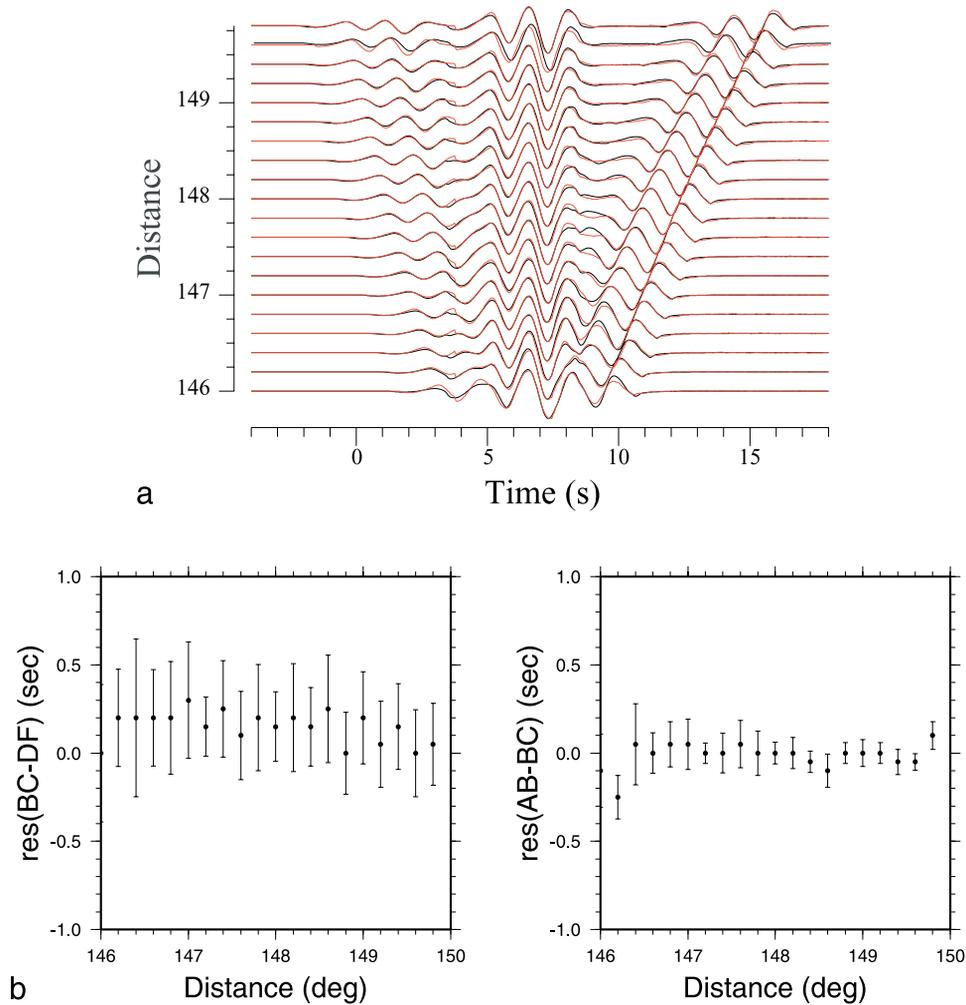
**Figure 6.** Nonlinear analysis of synthetic *PKP* data computed with the WKBJ software for an earthquake at 610 km depth. (a) WKBJ synthetic seismograms (black lines) and synthetic seismograms predicted by the best model (red lines) aligned on the *PKP*(BC) phase. (b) BC-DF and AB-DF best model residuals as a function of epicentral distance.
