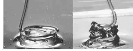
FIG. 4. Coexisting coiling states in an experiment with \nu=300 \text{ cm}^2 \text{ s}^{-1} , Q=0.041 \text{ cm}^3 \text{ s}^{-1} , d=0.15 \text{ cm} , and H=4.5 . (a) Low-frequency state; (b) high-frequency state.
