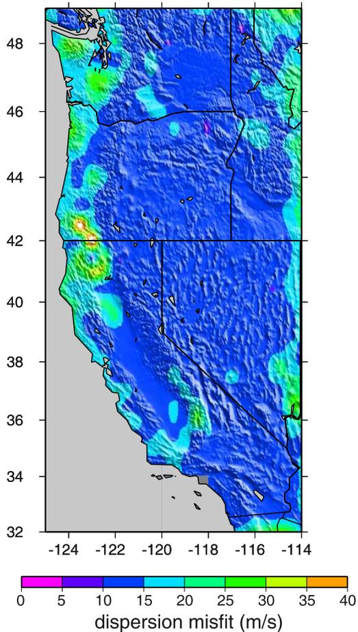
**Figure 4.** Period-averaged misfit map presenting the average of the difference between the observed dispersion curves and the curves computed from the 3-D  $V_s$  model. The largest misfit occurs west of the Cascade Range where the ambient noise and multiple plane wave earthquake tomography are most discordant in the period band of overlap (Figure 3f).
