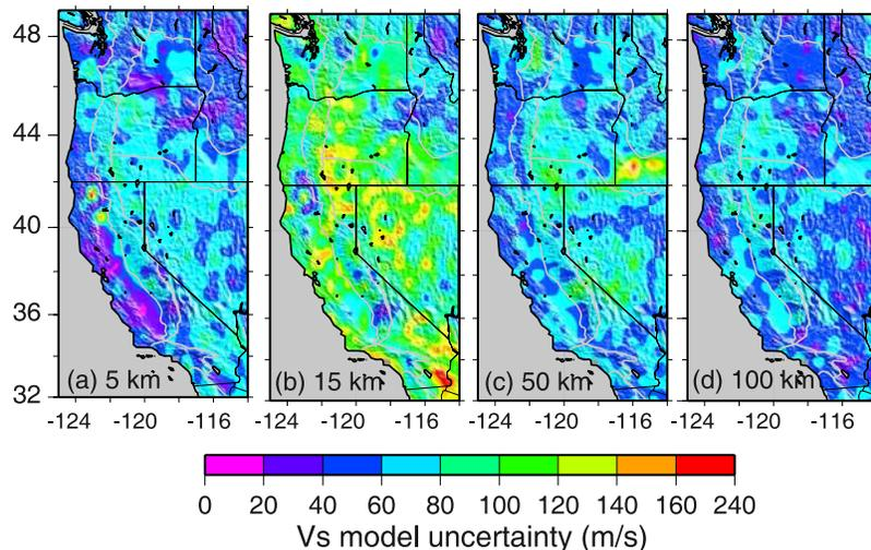
**Figure 6.** Maps of the estimated uncertainty of the 3-D  $V_s$  model derived from the ensemble of acceptable models produced by the Monte Carlo inversion at the depths of (a) 5, (b) 15, (c) 50, and (d) 100 km. The largest uncertainties are in the lower crust and uppermost mantle due to the trade-off between Moho depth and  $V_s$  in adjacent layers.
