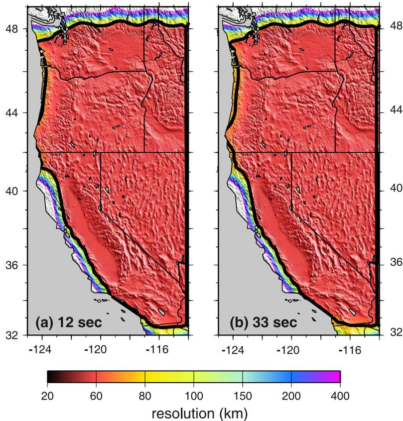
**Figure 2.** Resolution maps from ambient noise tomography for Rayleigh wave phase speed at periods of (a) 12 and (b) 33 s. Resolution is defined as twice the standard deviation of a 2-D Gaussian function fit to the resolution matrix at each point [Levshin *et al.*, 2005]. The 70 km resolution contour is shown with a thick black line. Resolution at other periods is similar.
