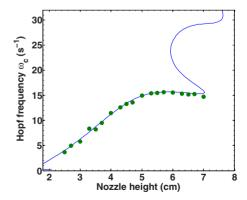
FIG. 7. (Color online) Measurements of the Hopf frequency  $\omega_c$  (solid circles) as a function of the nozzle height H. The solid line is the theoretical result from the linear stability calculation of Ref. [16]. The reversals in the theoretical curve mark the multifrequency regime.
