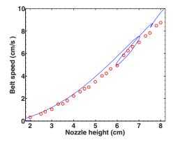
FIG. 5. (Color online) The critical belt speed  $U_c$  vs H, extracted from fits to amplitudes like the one shown in the previous figure. The solid line is calculated from the linear stability analysis of Ref. [16], with no adjustable parameters.
