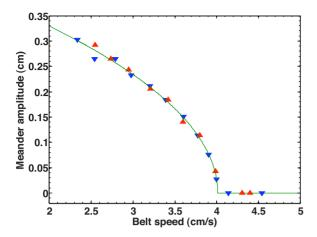
FIG. 4. (Color online) The amplitude |A| of the meandering motion as a function of the belt speed U, for H=5.3 cm. The upward (downward) pointing triangles indicate data taken with increasing (decreasing) U. The solid line is a fit to Eq. (4) with  $U_c$  =4.01 cm/s and  $\mu$ =4.62 cm<sup>-2</sup>. No higher-order terms were required. The smallest nonzero amplitudes here are about half the width of the thread.
