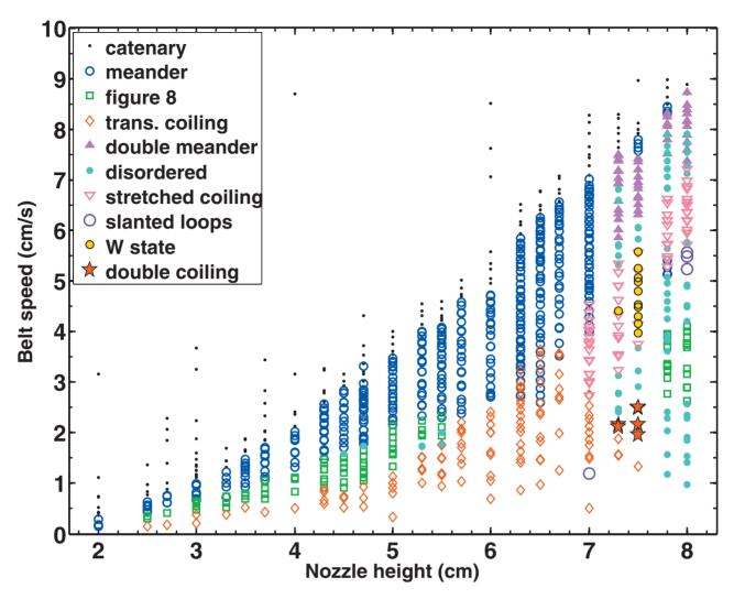
FIG. 3. (Color) The state diagram, as a function of the belt speed U and the nozzle height H. Some of the simpler states are shown in the previous figure; more complex states are described in Ref. [15].
