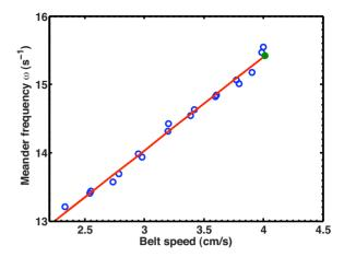
FIG. 6. (Color online) The angular frequency  $\omega$  of the meandering motion (open circles), as a function of the belt speed U, for H = 5.3 cm. The solid line is a fit to a linear variation of  $\omega$  vs U, consistent with a Hopf bifurcation. The solid circle marks the extrapolation to the critical value  $\omega_c$ .
